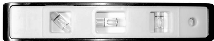
Figure 10-2-1. Level condition is read with the center vial.
