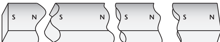
Figure 11-3-7. Magnetic poles in a broken magnet.
