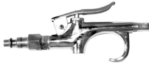
Figure 10-4-2. Most blow guns have nozzles that limit discharge pressure to 30 p.s.i.
