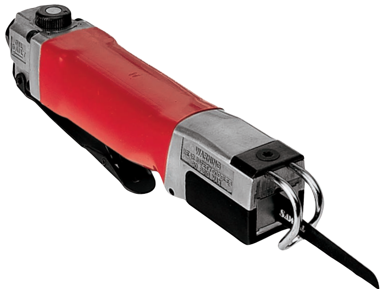
Figure 10-4-6. Air-powered sabre saws are lightweight and reduce the fire/explosion hazard. Photo courtesy of Snap-on Tools
