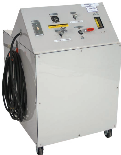
Figure 13-7-2. Portable hydraulic test stand.
