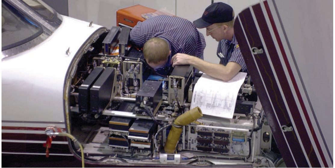
Figure 15-3-2. In a progressive inspection system, the complete inspection is broken down into sections. Each section comprises an inspection period. Photo courtesy of Duncan Aviation
