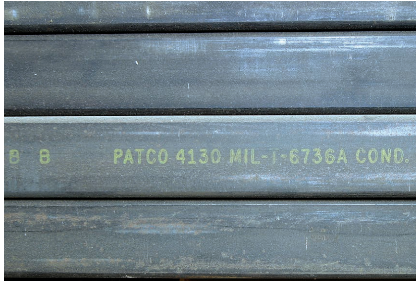
Figure 6-7-11. This pallet of steel tubing is marked with its four-digit number and with the heat-treat condition.
