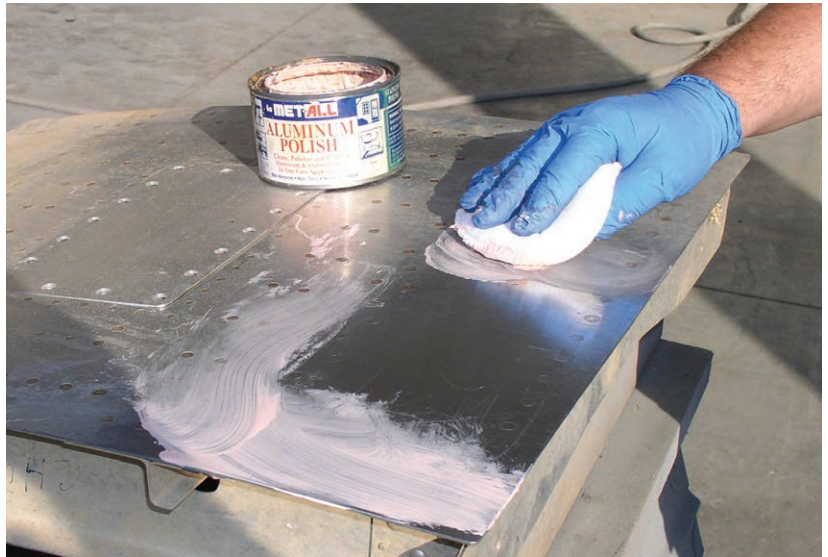
Figure 7-5-3. Hand-polish Alclad surfaces.
