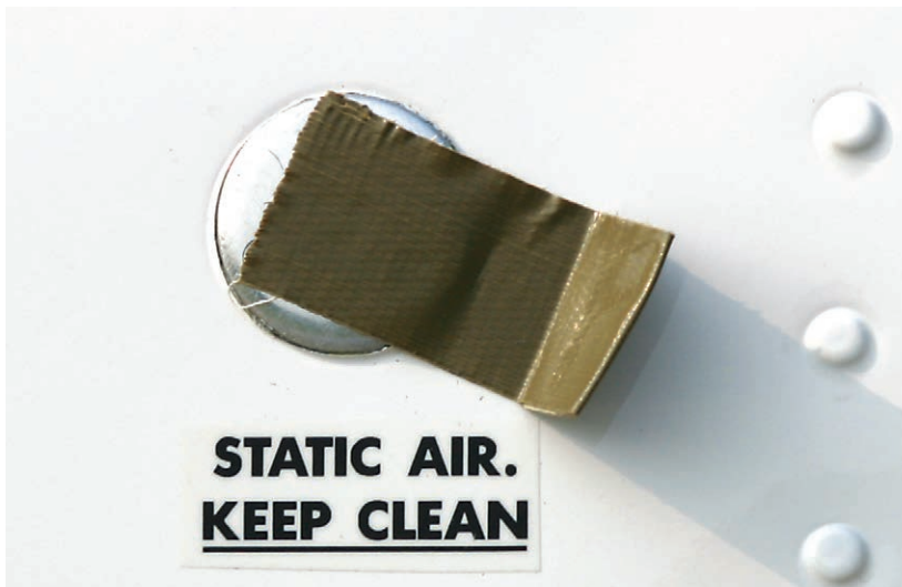
Figure 7-7-1. When taping a flush static port, fold back a piece of tape against itself. When applied, it will have a small tab that can be used to remove it. This also makes the taping more noticeable and harder to miss when time for removal.
