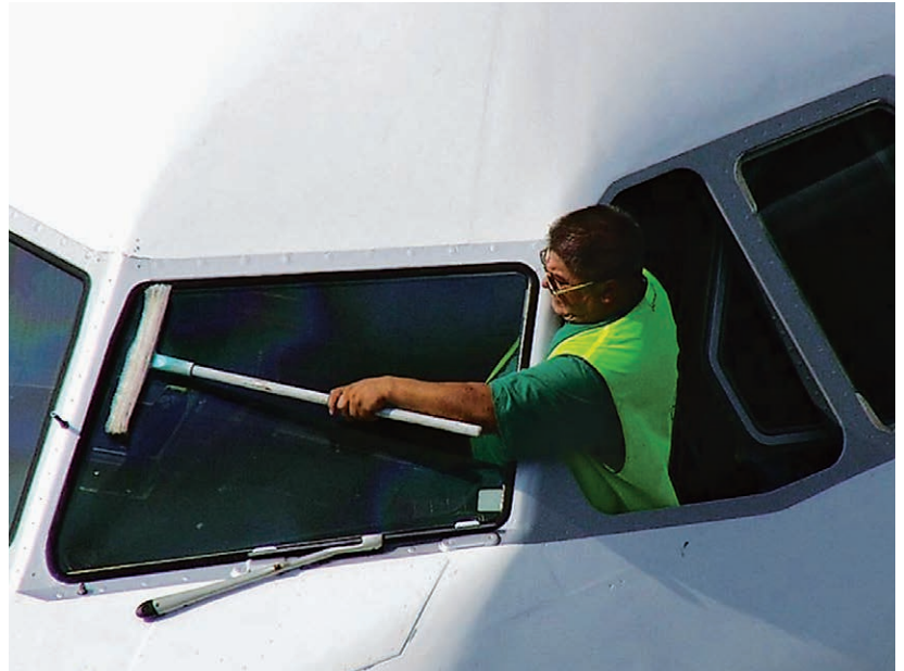
Figure 7-7-4. Cleaning an aircraft's windshield requires great care—use of a dusty cloth or marred implement will result in fine scratches and markings all over the surface being cleaned.
