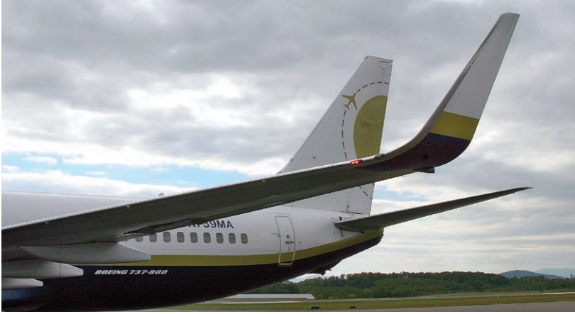
Figure 4-6-13. Winglets add considerable weight and structural complexity but do provide excellent drag reduction.
