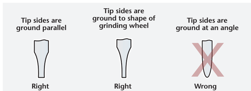
Figure 10-3-12. Screwdriver tip grinding.
