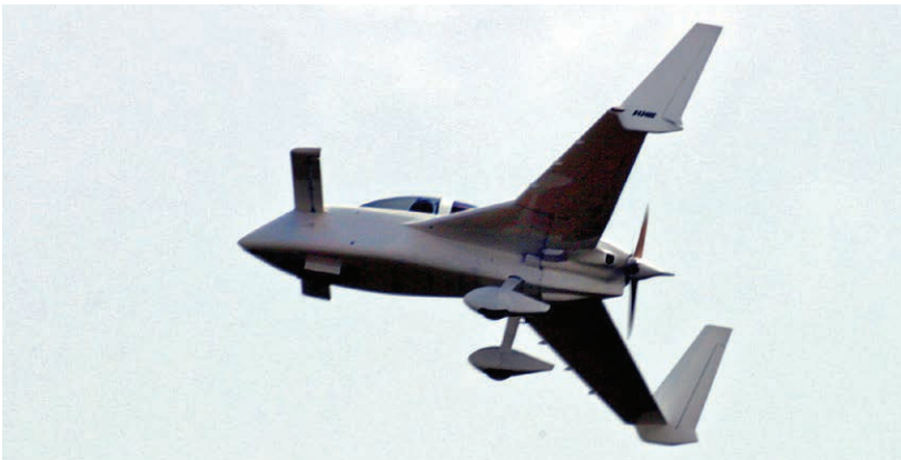
Figure 4-6-14. The Cozy series of homebuilt airplanes is currently one of the most popular examples of a canard design.
