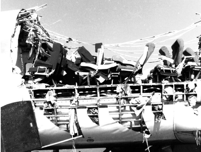
Figure 15-4-1. The Aloha Airlines mishap focused the need for improved corrosion inspections and an aging fleet inspection process.
