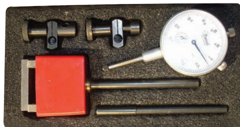
Figure 9-2-12. Standard dial indicators, using mounting adaptors, can be used to measure crankshaft runout.
