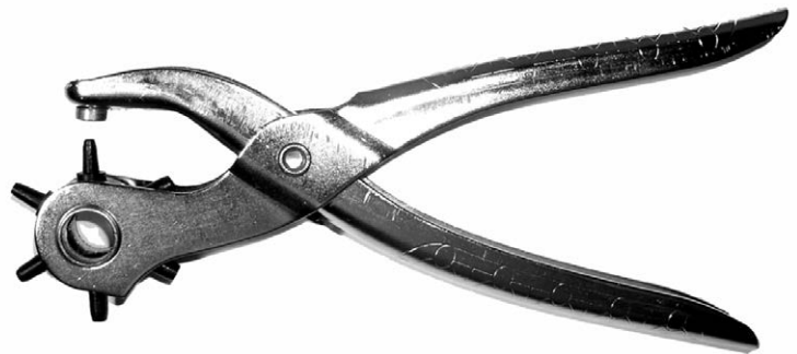
Figure 10-6-15. A leather punch has a range of hole sizes it can punch.
