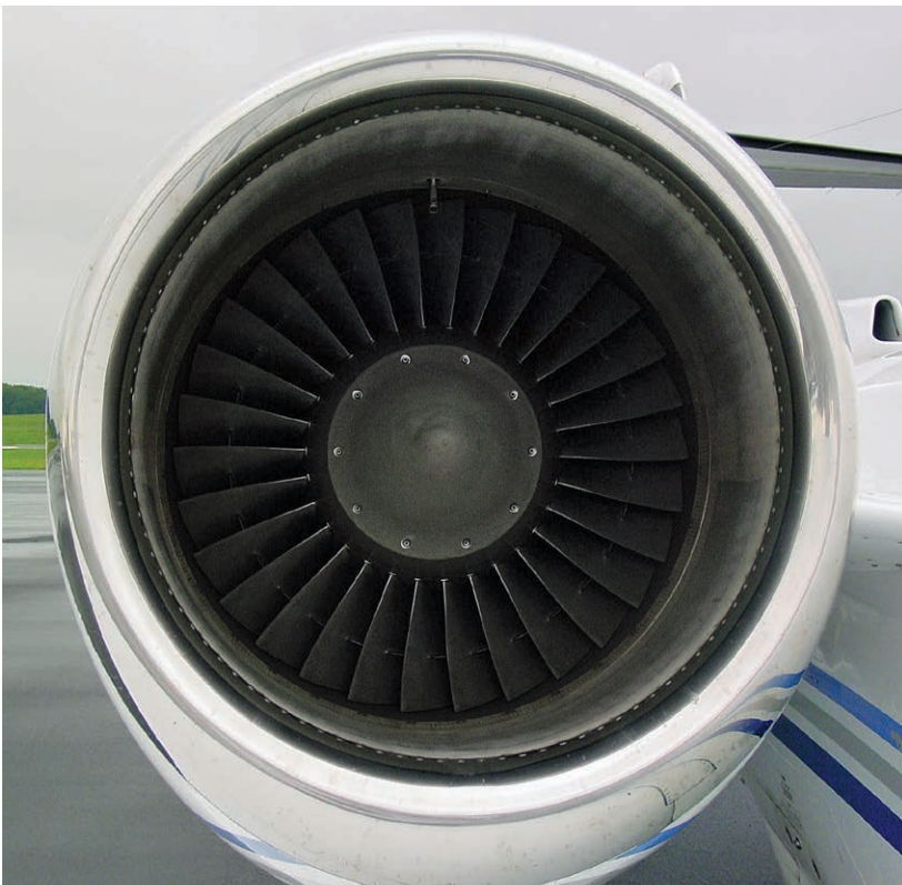
Figure 4-8-10. This nacelle shows off the airplane's inlet and diffuser, which slows airflow into the turbine engine. An aircraft's inlet design is based on the Bernoulli principle: As the air moves into the nacelle, the diffuser widens, which slows the speed of the air entering the compressor by raising the air pressure and lowering its velocity.
