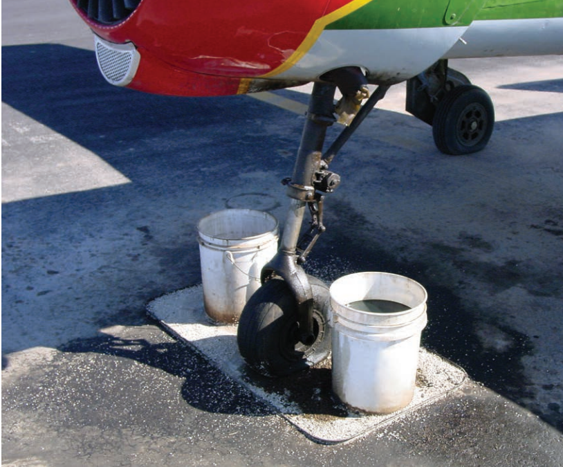
Figure 7-7-2. Engine oil leaks can make a real mess of a tricycle-geared airplane. Oil leaks can also shorten the life of the nose-wheel tire.
