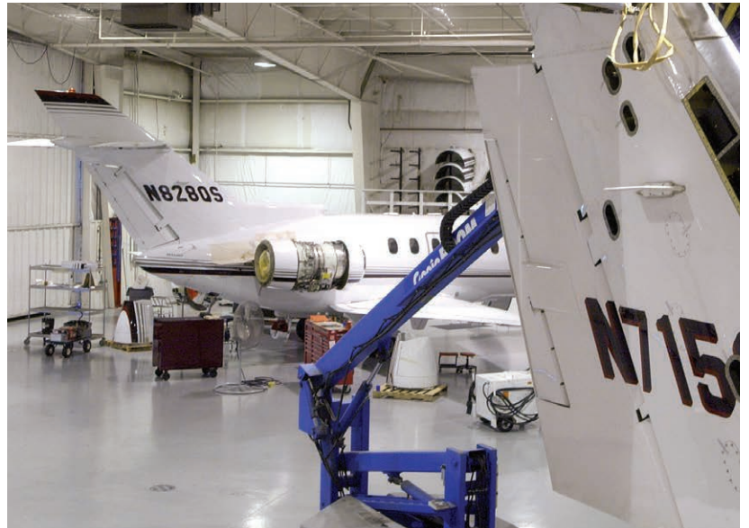
Figure 15-4-2. The use of platforms and lifts is necessary to access specific areas of some aircraft for inspection and repair. Photo courtesy of Duncan Aviation
