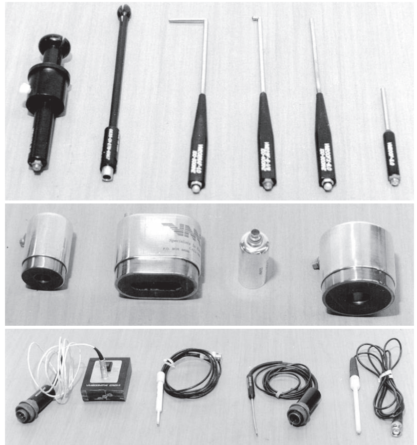
Figure 9-3-14. A sample of different eddy current test probes.
