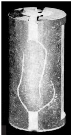
Figure 9-3-35. MPI of quenching cracks, shown with dry powder.
