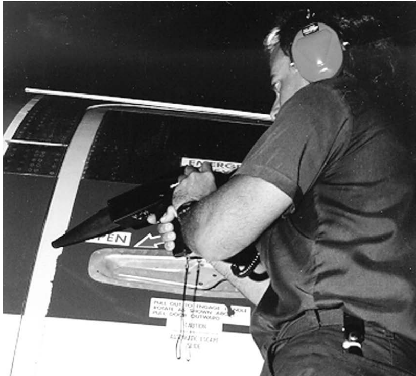
Figure 9-4-4. A maintenance technician checks a pressurized cabin for leaks. Photo courtesy of UE Systems, Inc., Elmsford, NY
