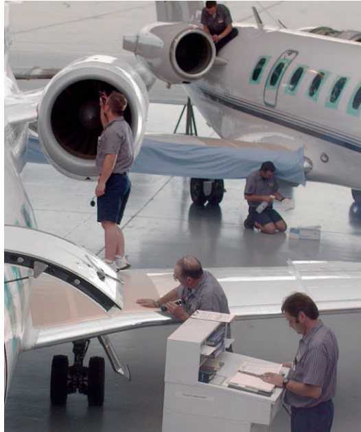
Figure 15-4-6. Teamwork is essential in today's shop environment. While most job cards cover a small segment of a given maintenance process, jobs must be accomplished in order, checked, and inspected. Photo courtesy of Duncan Aviation
