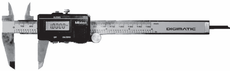
Figure 10-2-22. Direct-reading digital calipers take all the guesswork out of interpreting a measurement reading.
