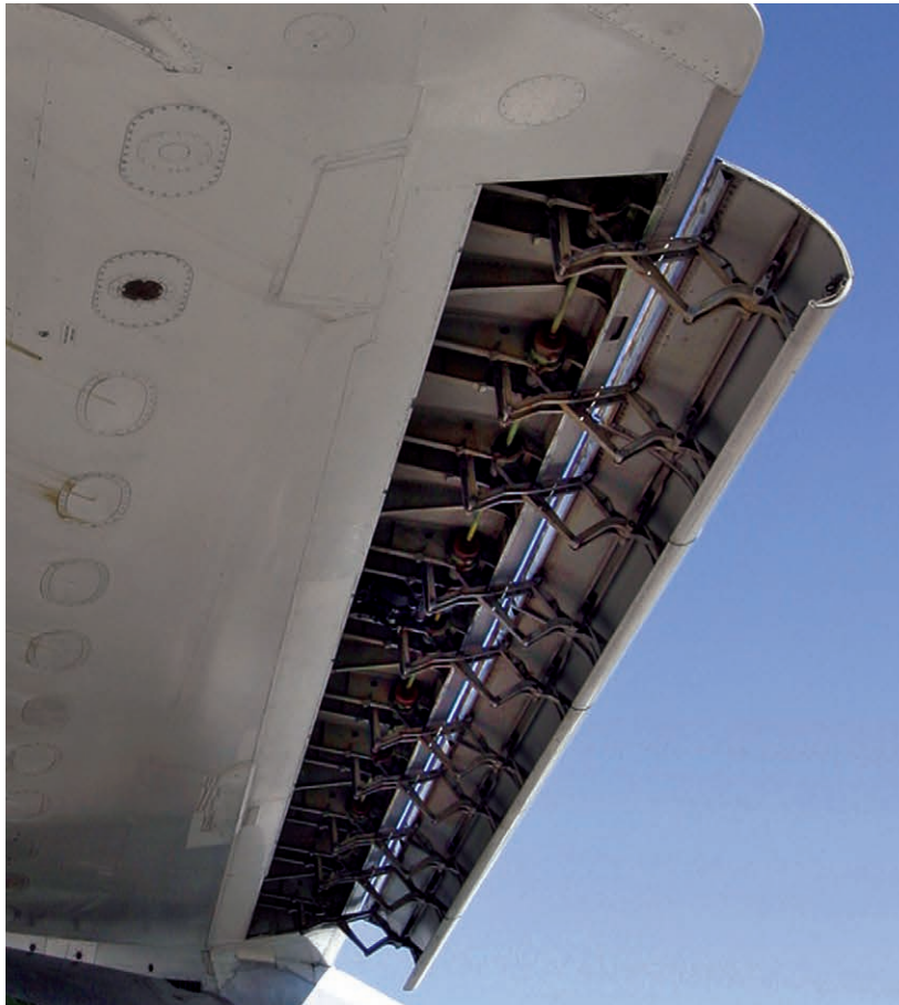
Figure 4-6-10. Leading-edge flaps on large transport airplanes can be quite complicated. By clever linkage design, this leading edge flap can unfold and extend, as in this view of a Kruger flap on a Boeing 747.
