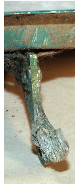
Figure 7-2-4. In this example the exfoliation is so advanced that the part is scrap.
