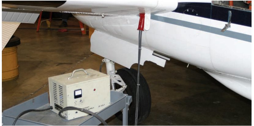
Figure 13-7-1. Benchtop-size APU supplies filtered DC to the airplane's ground power plug.
