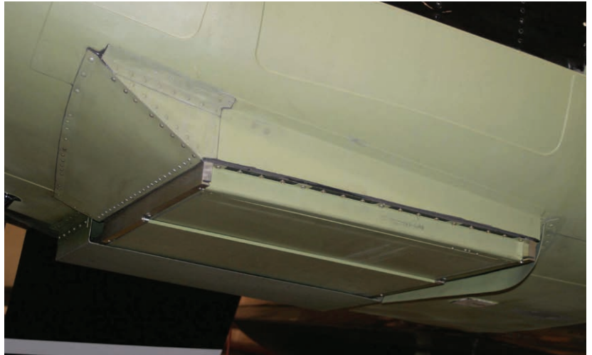
Figure 15-3-1. This camera hatch is certainly a major alteration. A modification of this type would likely require the services of a DER (Designated Engineering Representative).
