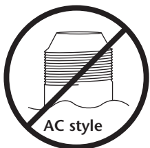
Figure 8-1-2B. AC fittings are no longer used.
