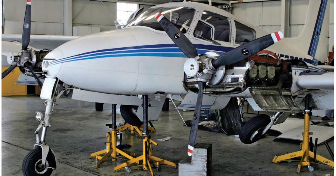
Figure 13-5-4. Tripod jacks are used to lift complete aircraft when gear retraction tests are required.
