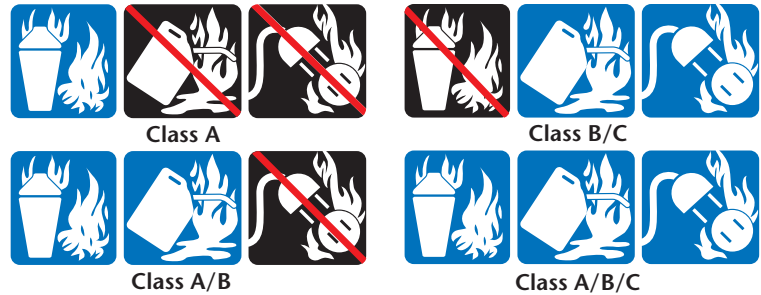
Figure 13-2-6. OSHA labels show how to define which extinguisher will work for what type of fire.
