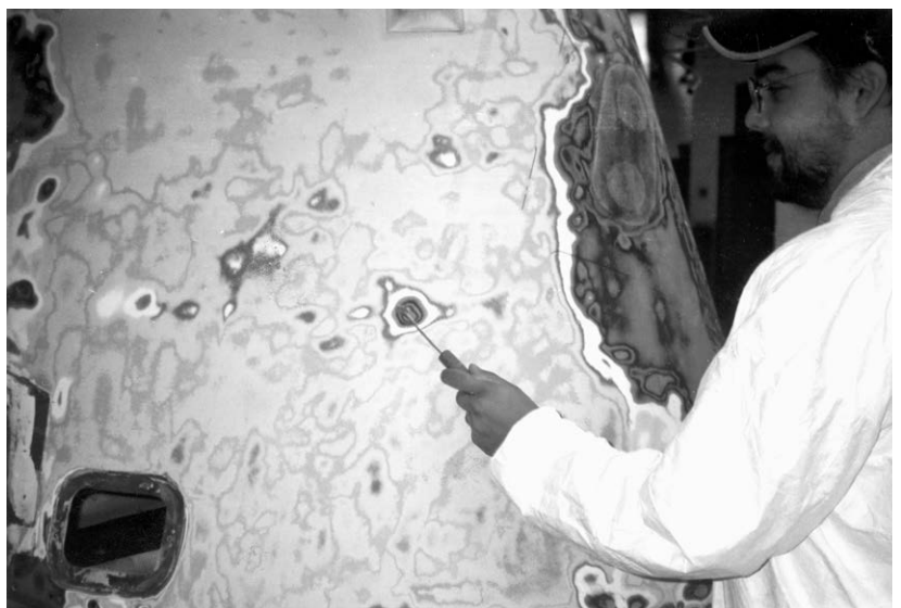
Figure 9-3-8. A composite technician tap tests a radome to detect delamination and disbond.
