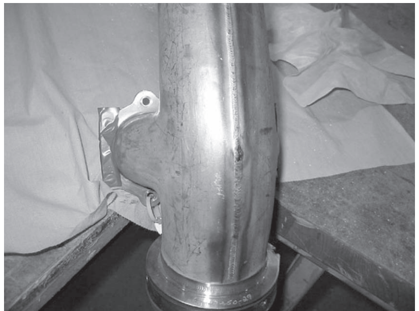
Figure 9-8-18. Welding often produces an undesirable heat treatment adjacent to the welded area.
