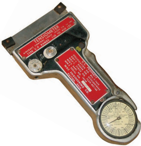
Figure 10-6-4. This type of aircraft cable tensiometer works for most general aircraft control systems.
