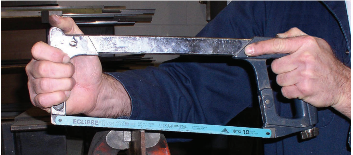
Figure 10-3-76. Proper way to hold a hacksaw.
