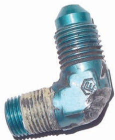
Figure 8-1-21. Fitting damaged by abrasion to the point it is unuseable.
