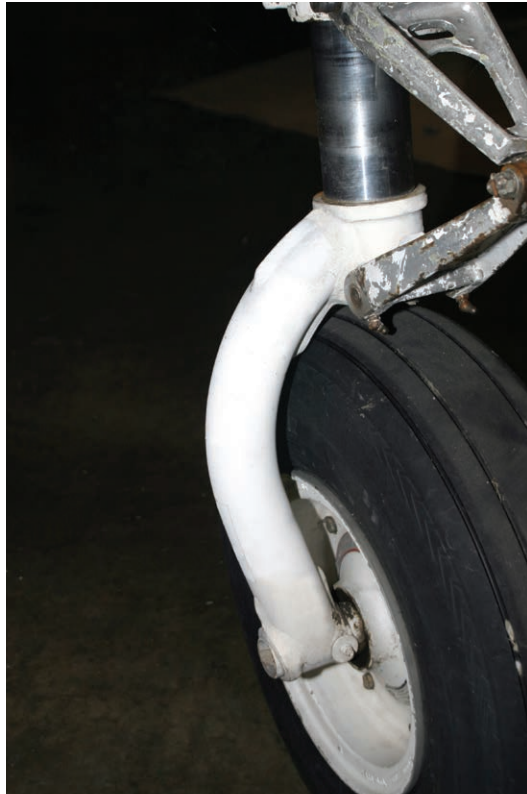
Figure 6-7-7A. This welded nose gear assembly, used on many Beechcraft King Air executive turboprops, is prone to cracking and is subject to a repetitive AD inspection.
