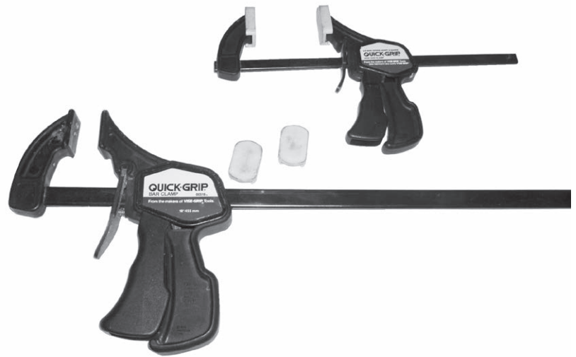
Figure 10-3-44. Adjustable bar clamps with rubber jaw pads.
