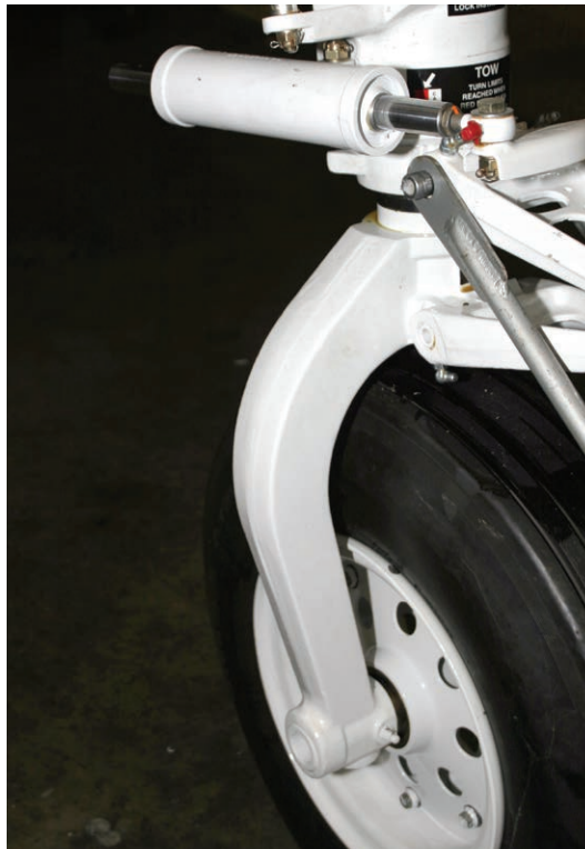
Figure 6-7-7B. The welded assembly has been replaced by this forged nose gear leg. The greater strength and predictable load bearing characteristics eliminate the need for a repetitive inspection.
