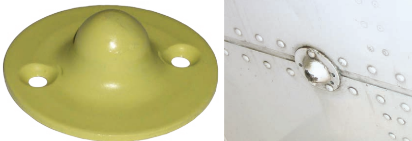
Figure 13-5-5. Two types of jack pads.
