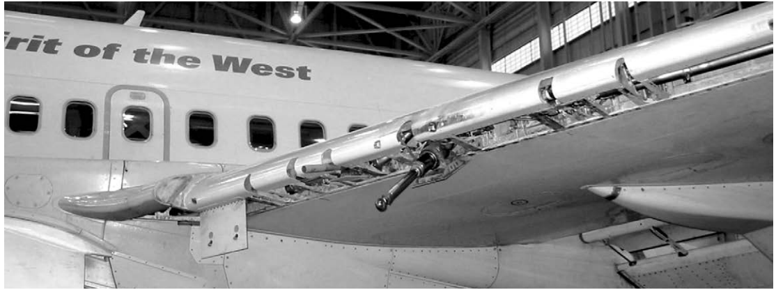
Figure 9-9-1. The leading-edge slat has been removed from the wing. Its reinstatement is a required inspection item.
