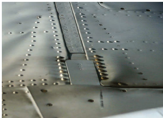
Figure 15-3-3. Severe turbulence can leave permanent wrinkles in wing skins.
