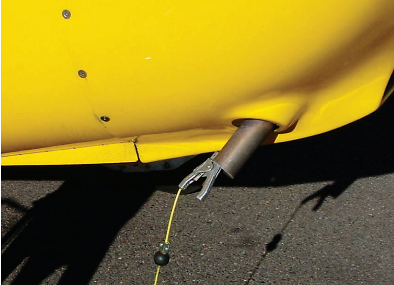
Figure 13-8-3. Do not use the engine exhaust or propeller as grounding points.
