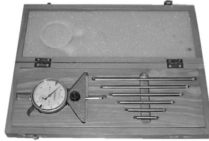
Figure 9-2-9. This depth micrometer set has interchangeable spindles that allow measurement of deep holes.
