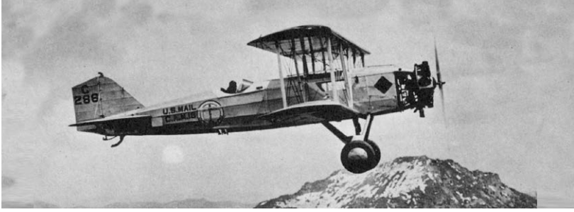
Figure 9-0-2. Aircraft Type Certificate No. 2 was issued to the Boeing 40A. It was the first transport-type aircraft certified under the new CAA rules.
