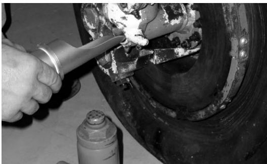
Figure 13-5-2. Many aircraft with an oleo-type strut have jack pads that insert into the hollow axle.
