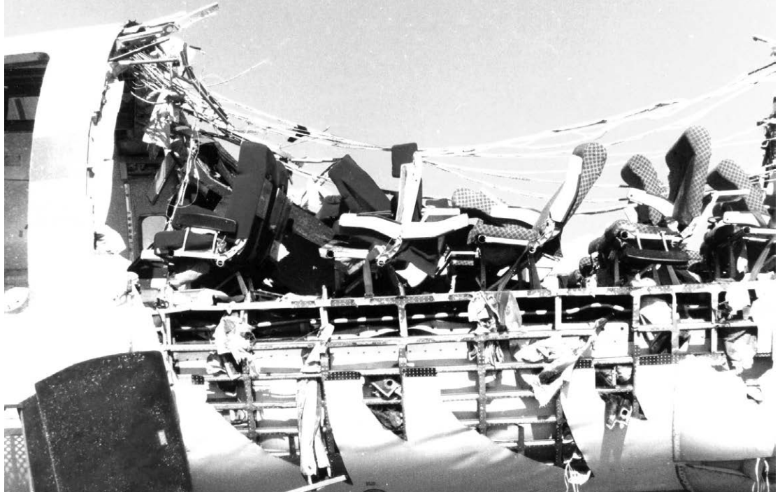
Figure 9-7-1. The structural failure of the upper cabin of an Aloha Airlines 737-200 was the event that put national focus on aging aircraft and corrosion inspections.
