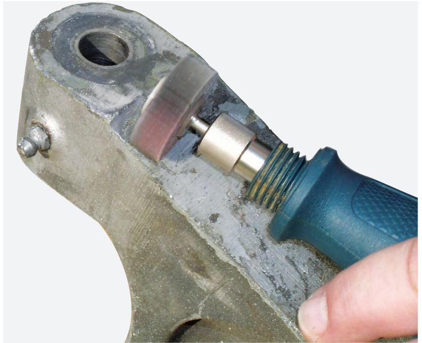
Figure 7-5-9. Careful removal of corrosion from a highly stressed magnesium part.
