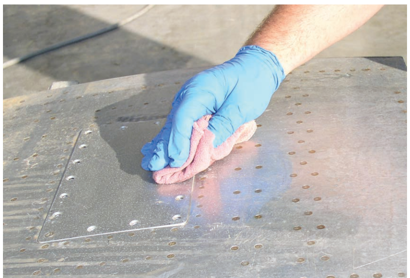
Figure 7-5-5. Dry the treated surface.
