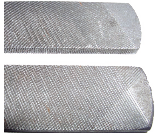
Figure 10-3-55. Single- and double-cut file teeth.
