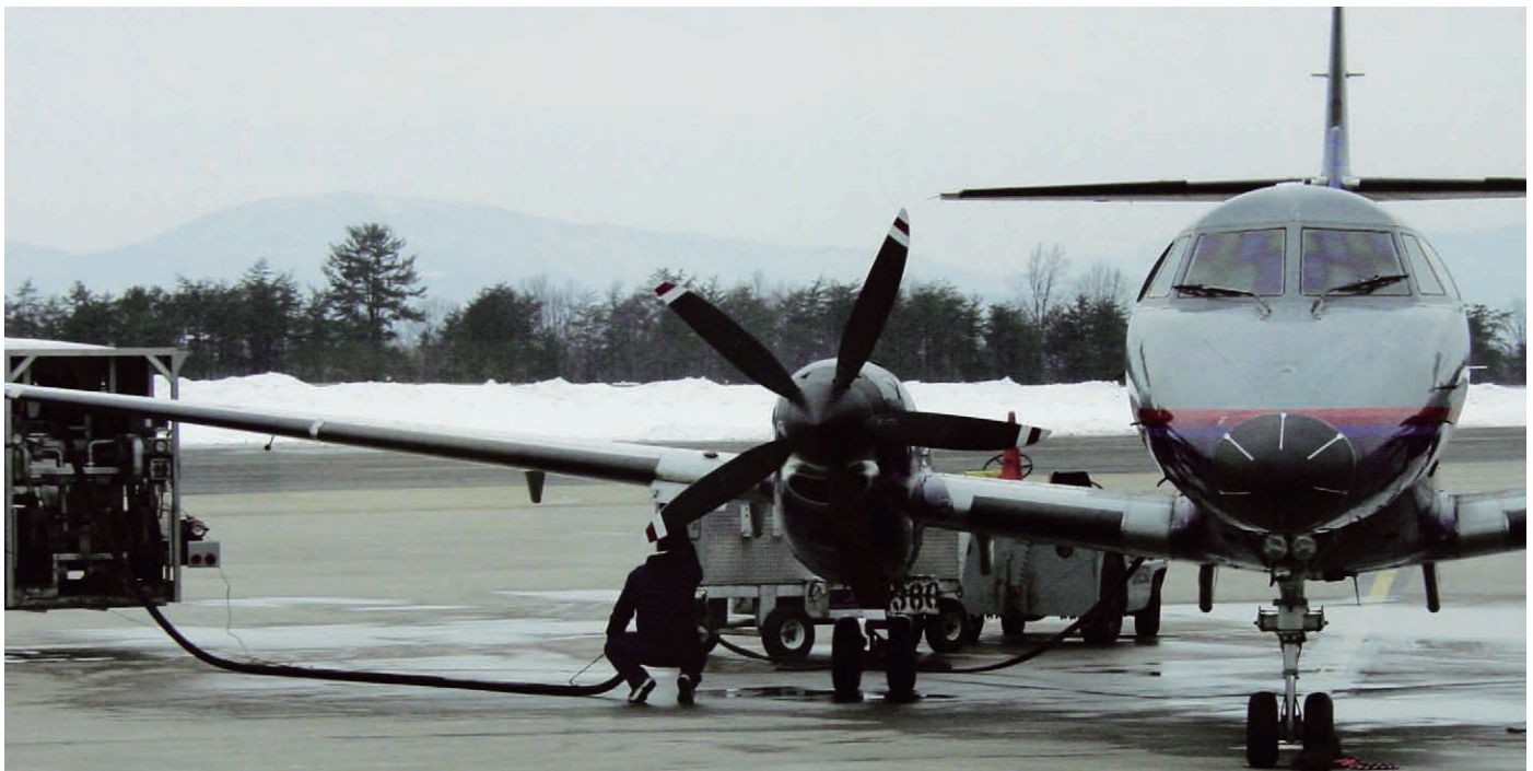
Figure 13-8-1. Pressure fueling system in use.
