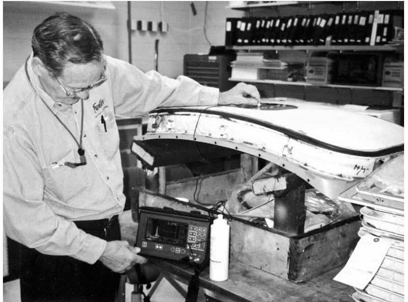
Figure 9-3-7. Standard practice allows aircraft maintenance technicians to polish out small cracks and pits in aircraft windows. Here an inspector uses an ultrasonic test unit to find the thickness of a repaired window in an emergency escape hatch.
