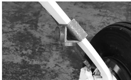
Figure 13-5-3. Spring steel landing gear legs must have special adaptors to allow jacking.
