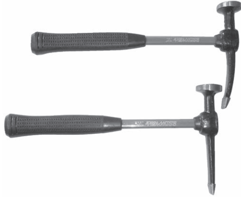
Figure 10-3-2. Body hammers are specialty tools used in the auto body trade. They are used principally for finishing hand-formed parts.
