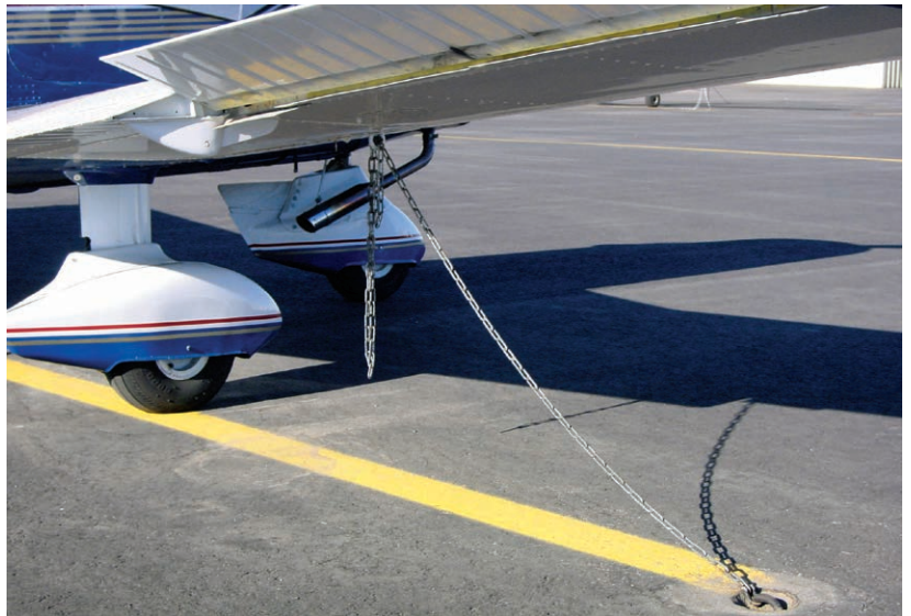
Figure 13-4-3. Properly connected, chain makes the best tiedown lead.
