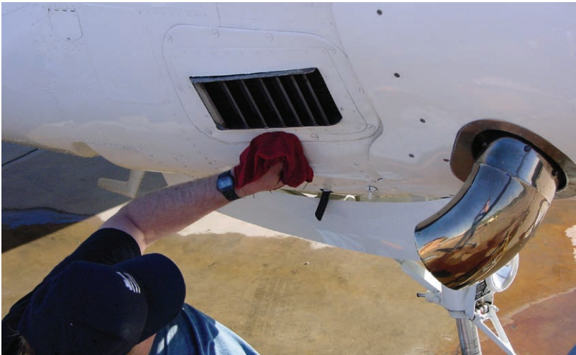
Figure 7-7-3. All airplanes leave an exhaust track somewhere on the structure. If not removed regularly, the stain will start corrosion of the structure from the combustion byproducts present.
