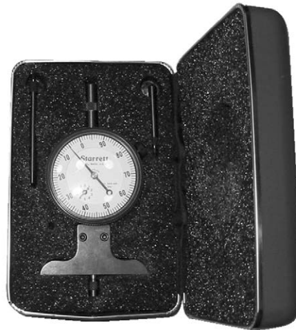
Figure 9-2-11. This dial indicator is ideal for measuring corrosion damage. Other dial indicator styles are used for measuring crankshaft and propeller shaft run-out.
