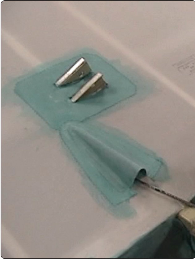
Figure 3-32. A strut fitting and cable guide with reinforcing fabric gussets cemented in place.
