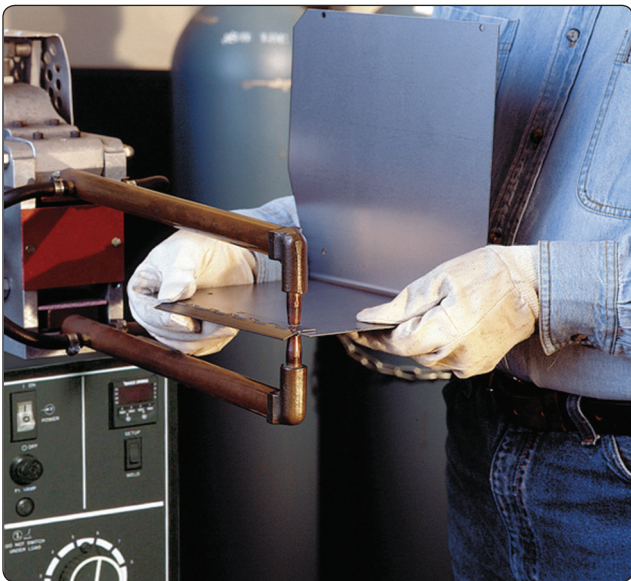
Figure 5-10. Spot welding thin sheet metal.
