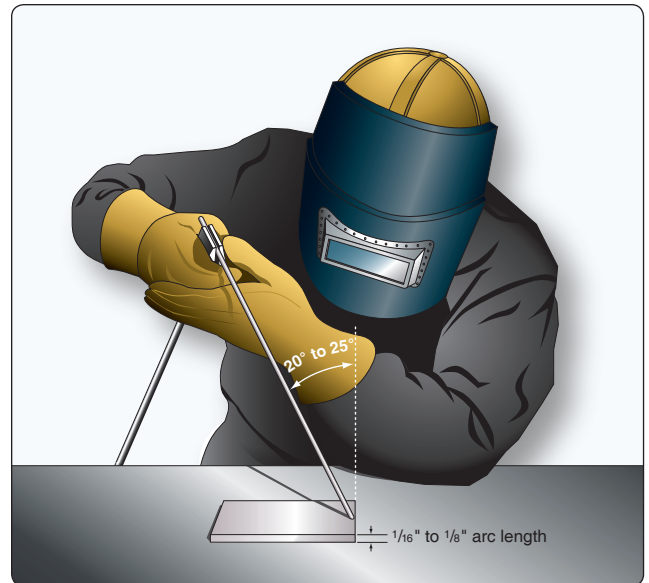
Figure 5-32. Angle of electrode.
