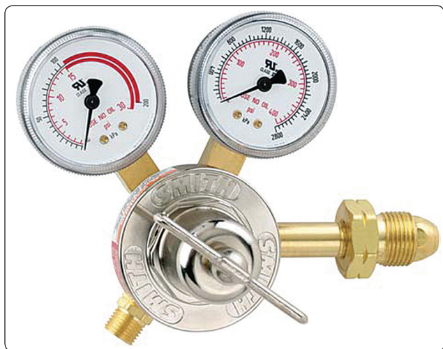
Figure 5-13. Single-stage acetylene regulator. Note the maximum 15-psi working pressure. The notched groove cylinder connection nut indicates a left-hand thread.
