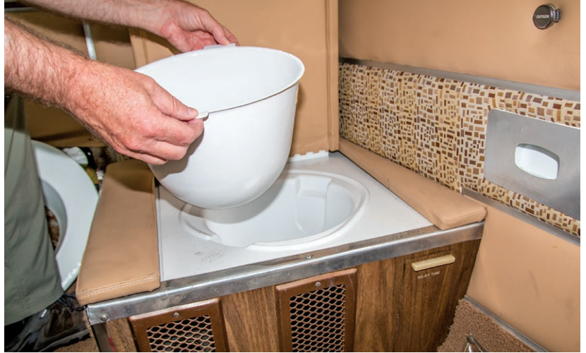
Figure 5. The canister can be removed for servicing.
