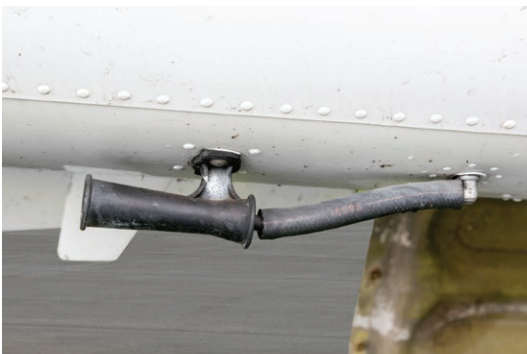
Figure 4. This relief tube is stowed under the pilot seat (top) and can be extended for relief (middle). The liquid exits via the venturi (bottom).
