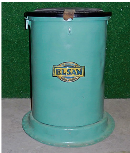
Figure 6. Elsans were used to store waste in World War II-era British aircraft. Courtesy of Bomber Command Museum of Canada
