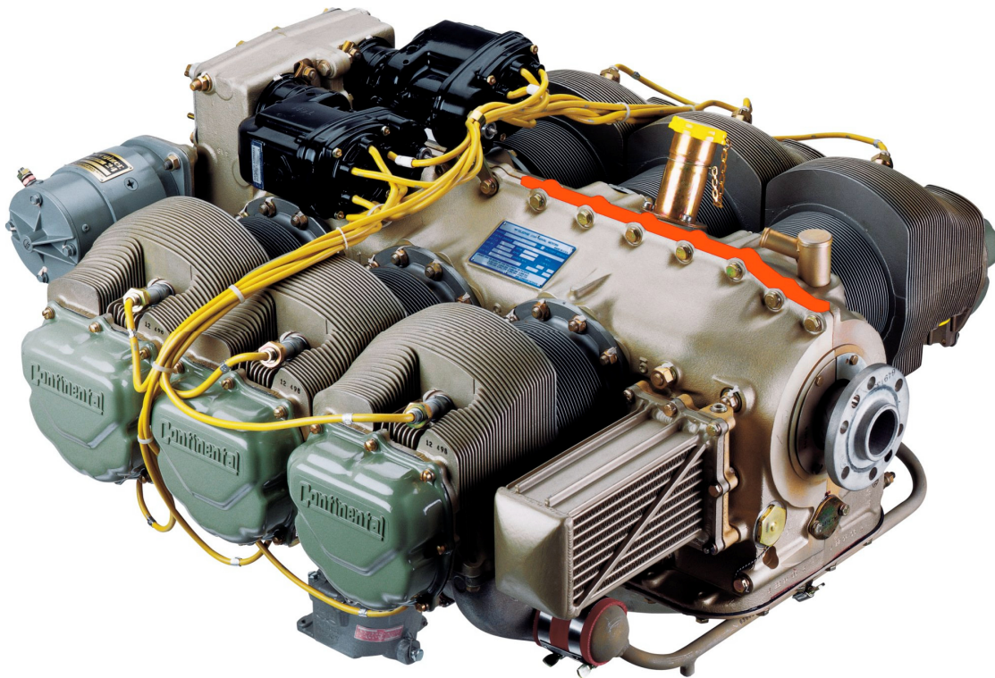
Figure 2-13. Sealant Applied to Backbone of Crankcase (Highlighted in Red)
