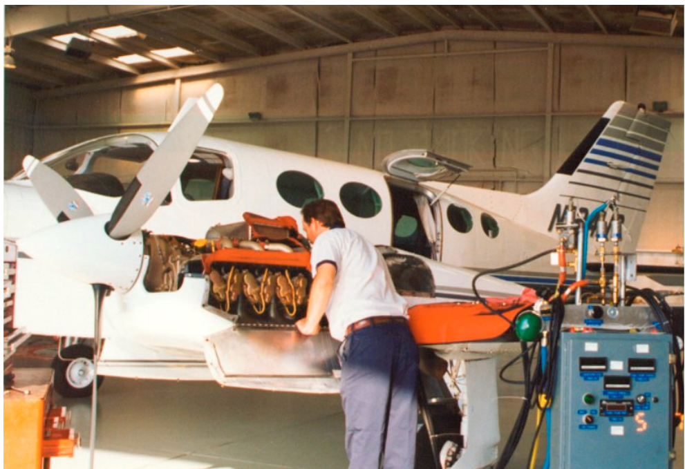
Setting up the Fuel Injection System
