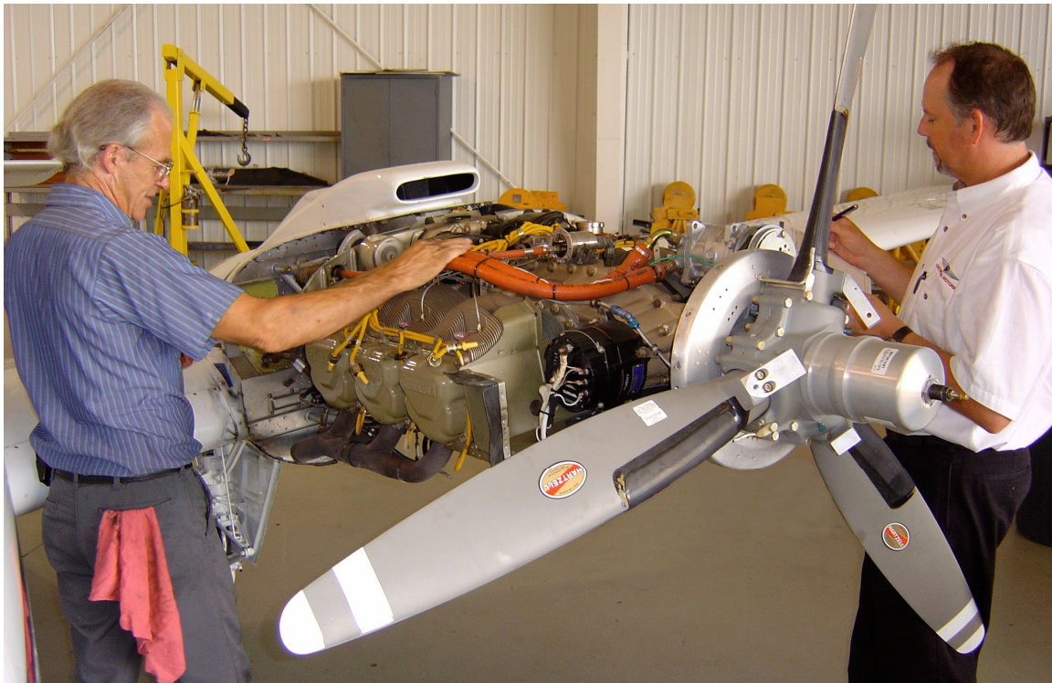
Inspecting Cylinders During an Annual Inspection
