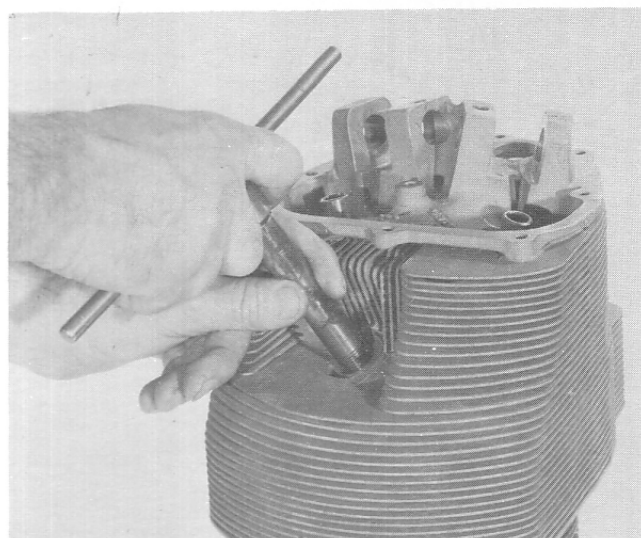
FIGURE 5-5. EXPANDING SPARK PLUG HOLE HELICAL INSERT.
