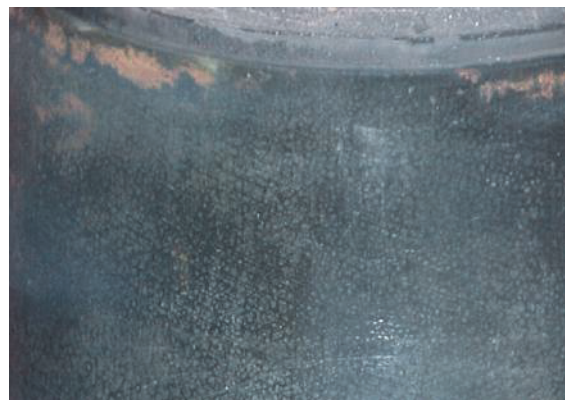
Figure 6-32. Phosphated Cylinder Bore
