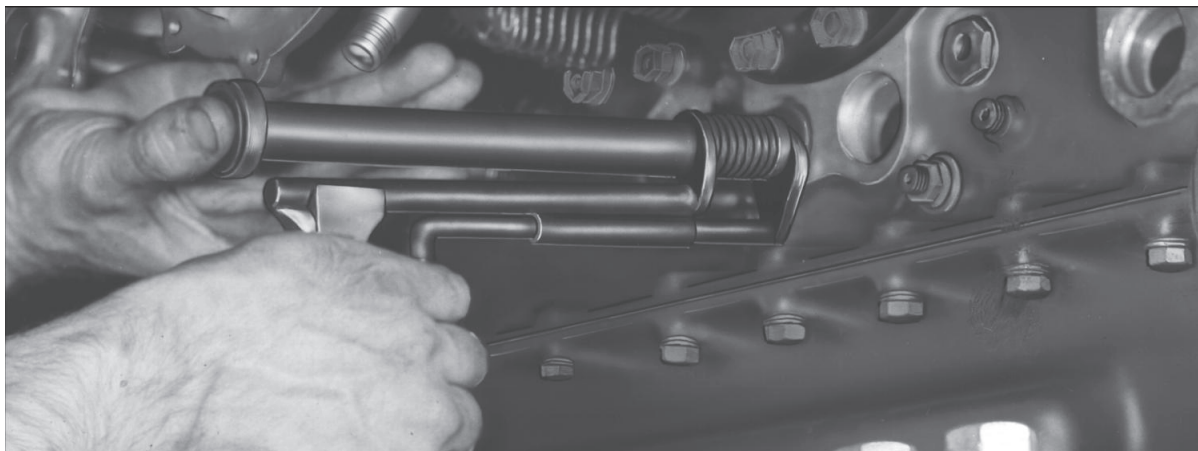
Figure 17-16. Pushrod Housing Installation
