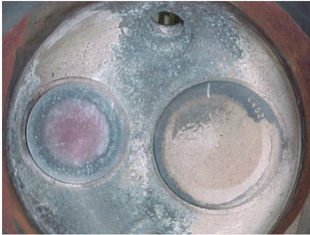
Figure 6-29. Normal Combustion Chamber
