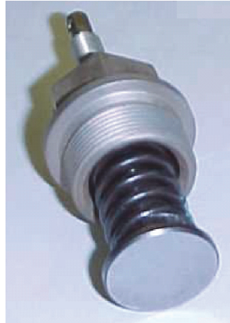
Figure 10-23. Oil Pressure Relief Valve
