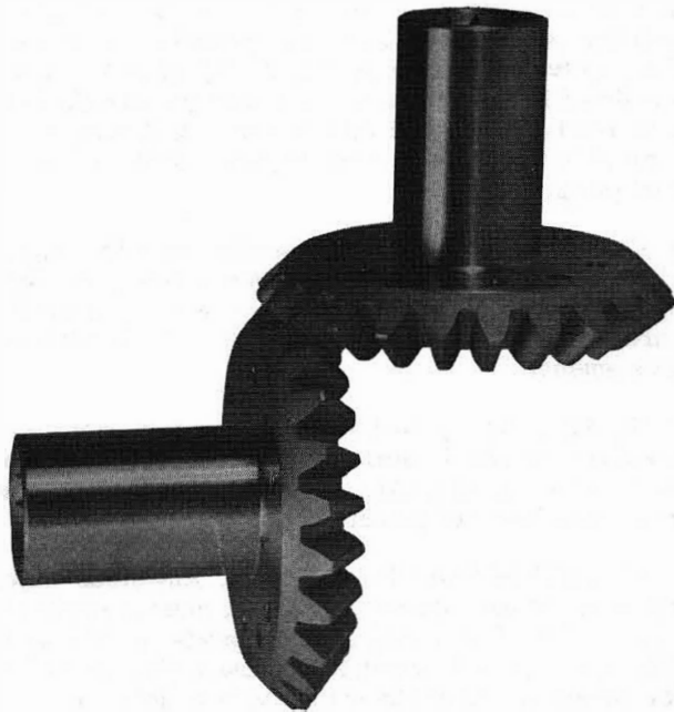
Figure 3-1. Bevel Gear - Showing Extreme Pitch Alignment
