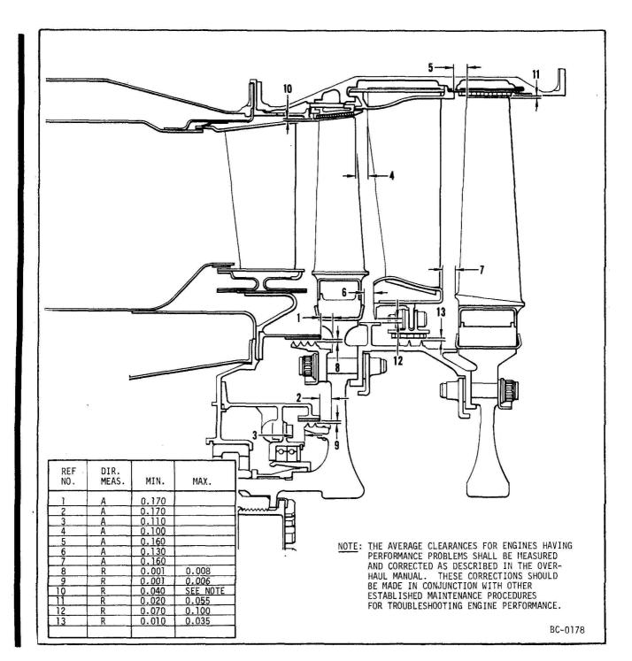
Turbine Section Clearances - CF700-2D and -2D-2 Figure 204A
