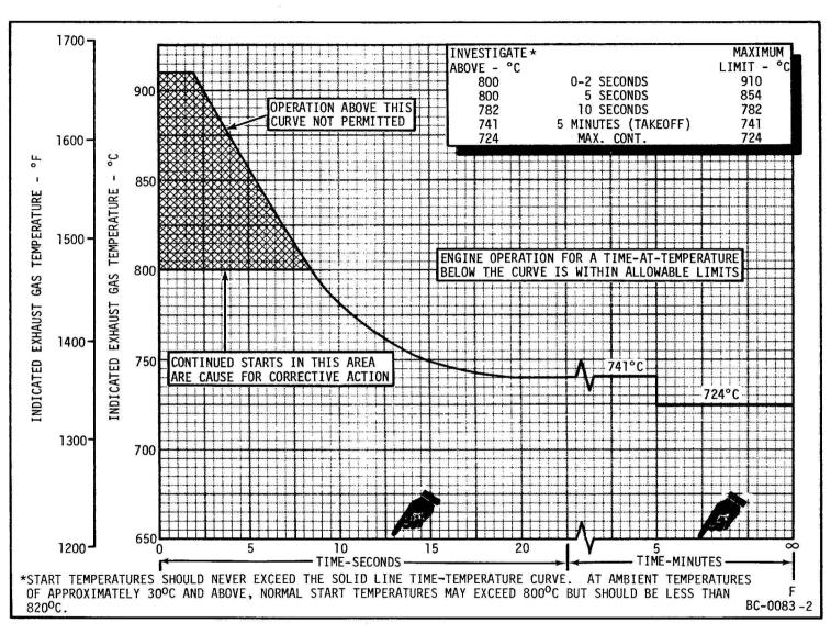
Exhaust Gas Temperature CF700-2D and -2D2 (Alternate Immersion Harness) Figure 504C CF700 TURBOFAN
