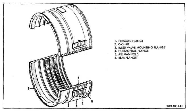
Compressor Casing Inspection Figure 201
