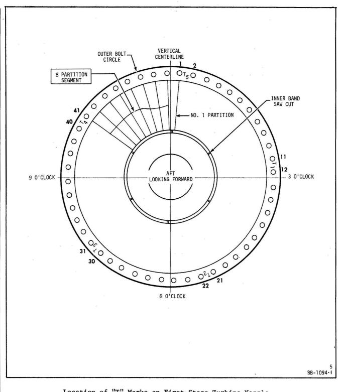
Location of "T" Marks on First-Stage Turbine Nozzle Figure 205
