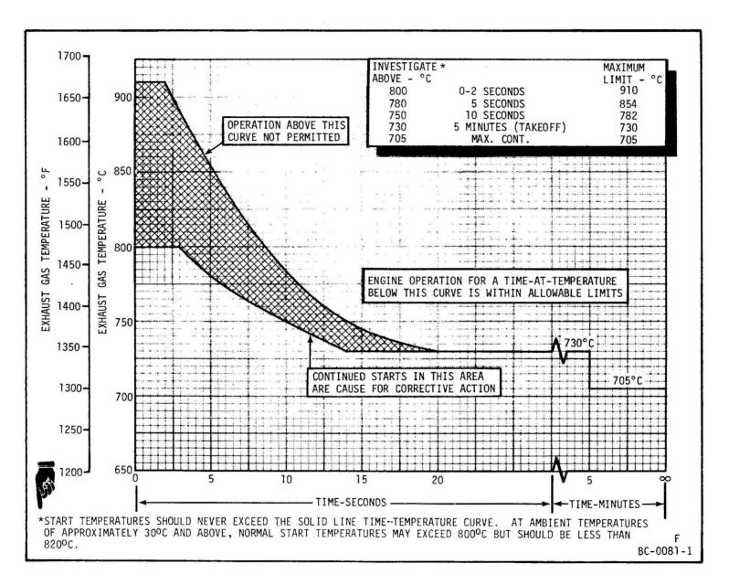
Exhaust Gas Temperature Limits CF700-2C (Aspirating Harness) Figure 504
