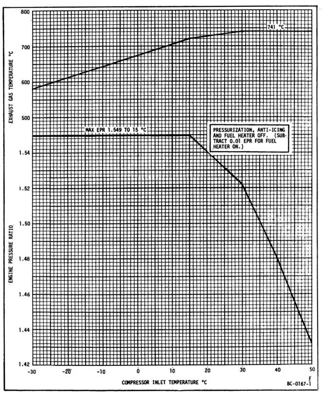
Power Assurance Check for CF700-2D-2 Engines Installed in Falcon Models 20E and 20F Aircraft (Engine Serial No.s 304325 and up, or Engines MODIFIED per Service Bulletin 72-128) Figure 509D
