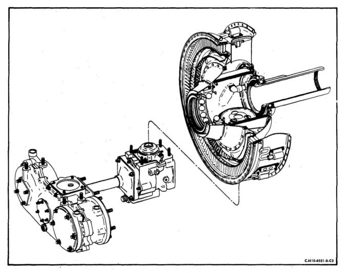
Accessory Drive Section Figure 1 MAINTENANCE MANUAL
