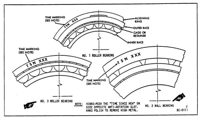
Time-Marking of Engine Bearings Figure 1
