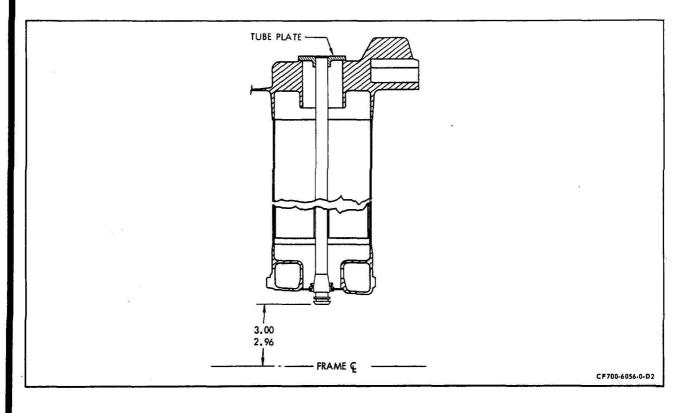
Sump Vent Tube Plate Replacement Figure 204
