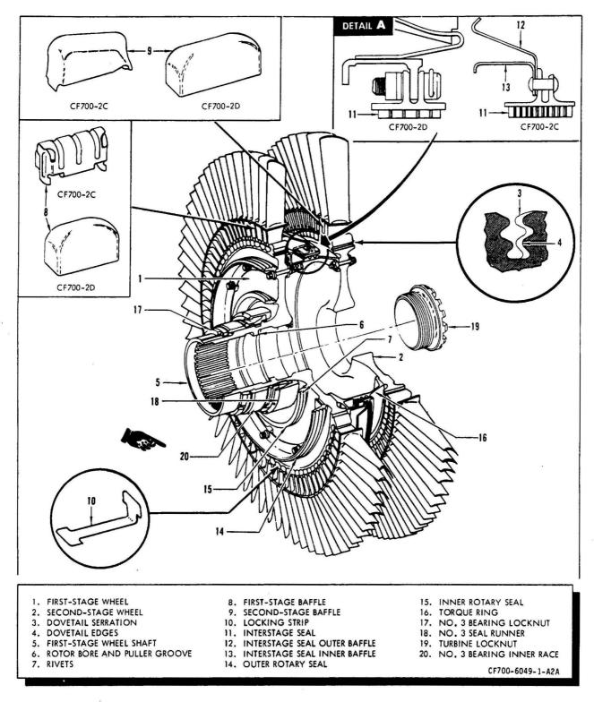
Turbine Rotor Assembly Figure 201
