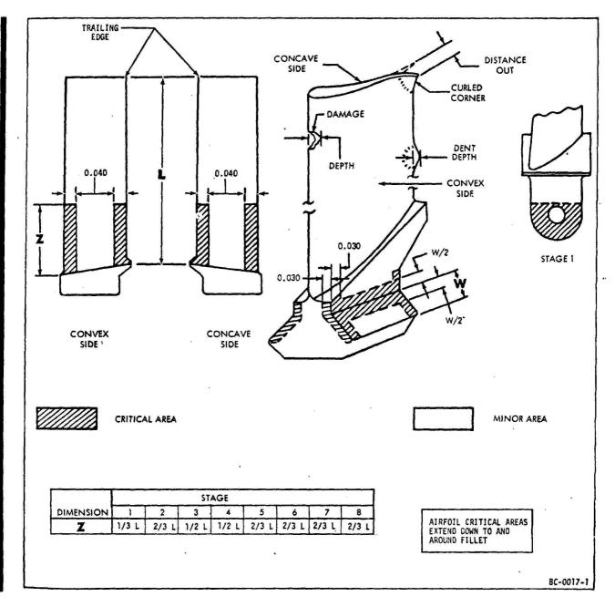
Compressor Rotor Blades - Inspection Figure 201
