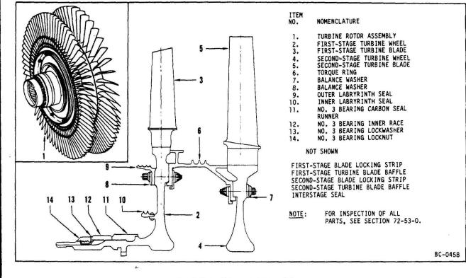
Turbine Rotor Assembly Figure 2 SEI-187
