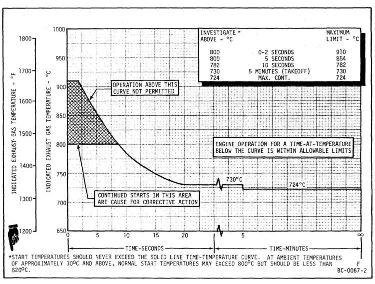
Exhaust Gas Temperature CF700-2C (Alternate Immersion Harness) Figure 504B
