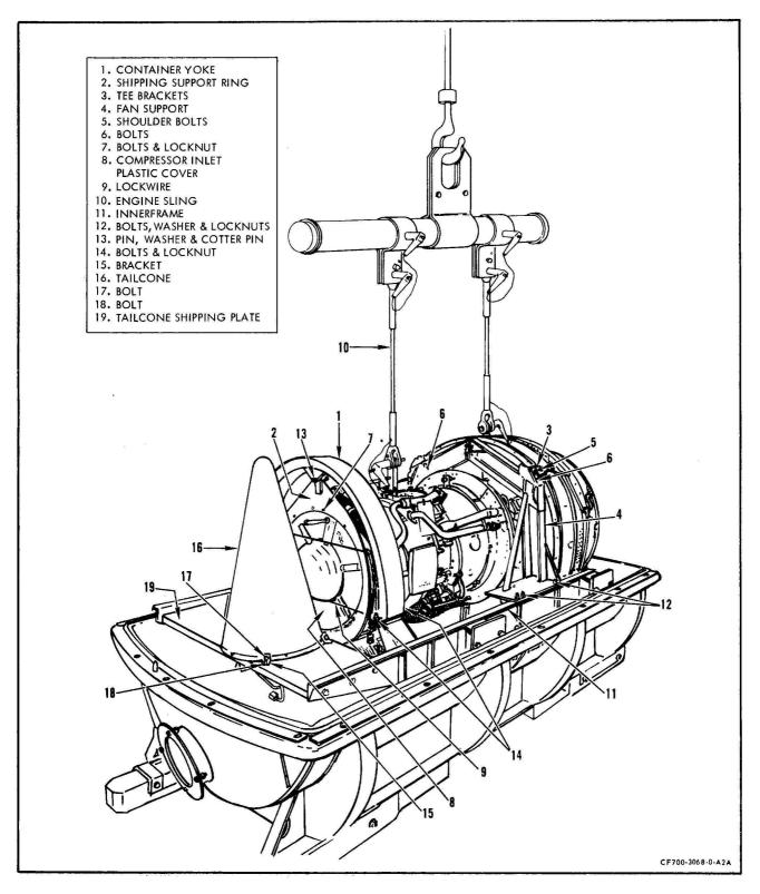
(13) Align holes of container yoke and inner frame. Insert 7/16-20 hex head bolts (14), threaded section of bolts must be in up position. Turn on locknuts until finger tight.
