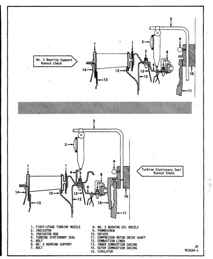
No. 3 Bearing Support and Turbine Stationary Seal Runout Checkout Figure 203 SEI-187
