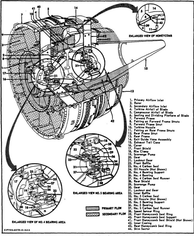
Aft Fan Section Figure 1 (Sheet 1 of 2)
