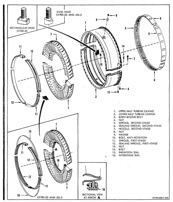
Turbine Stator Assembly Figure 201
