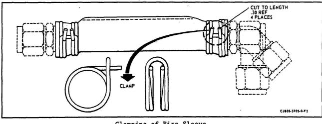
Clamping of Fire Sleeve Figure 3
