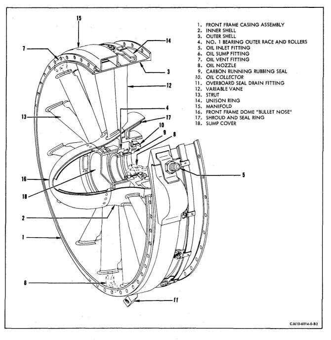
Front Frame Assembly Figure 1 Т
