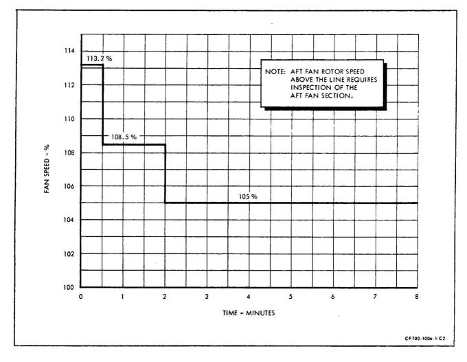
Aft Fan Transient Overspeed Limits Figure 508
