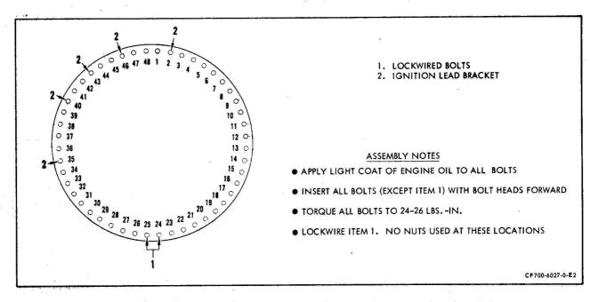
Outer Combustion Casing - Mainframe Flange Bolt Circle Figure 202
