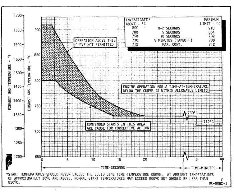
Exhaust Gas Temperature Limits CF700-2D (Aspirating Harness) Figure 504A CF700 TURBOFAN
