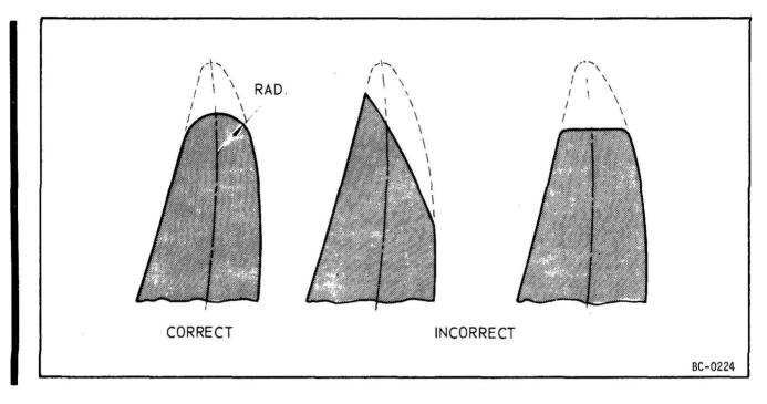
Typical Leading Edge After Blending Figure 205 MAINTENANCE MANUAL
