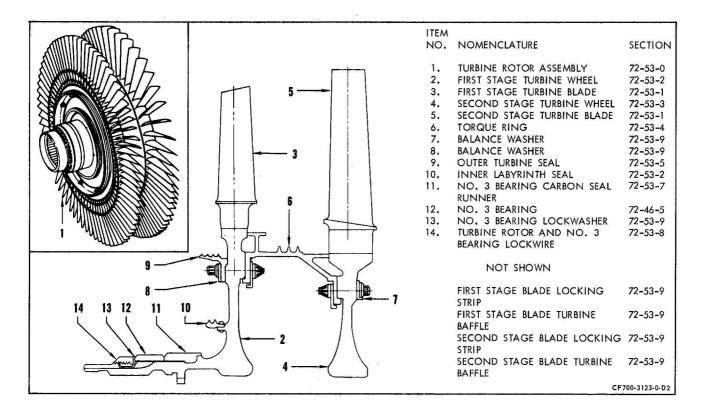
Turbine Rotor Assembly Figure 2 SEI-187
