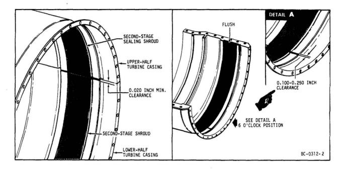
Second-Stage Turbine Shrouds - Installation CF700-2C Figure 203A
