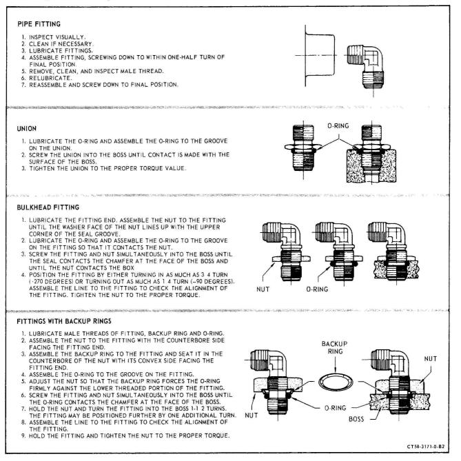
Assembly Procedures - Hose and Tube Fittings Figure 1
