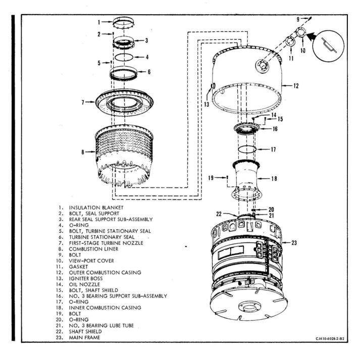
Combustion Section - Installation Figure 201
