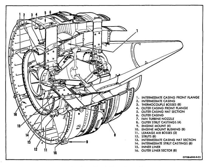
Fan Section - Front Frame Inspection Figure 202
