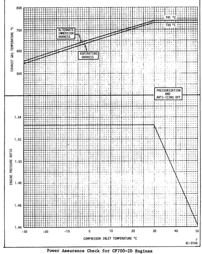
Installed in Falcon 20D Aircraft Figure 509B
