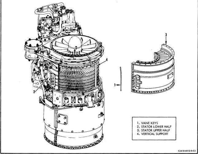
Compressor Stator Upper Half Removal Figure 202
