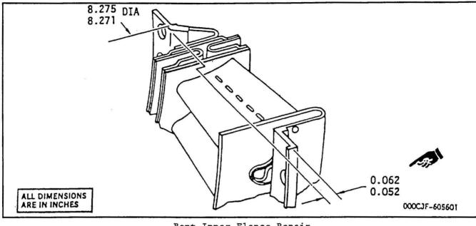
Bent Inner Flange Repair Figure 203
