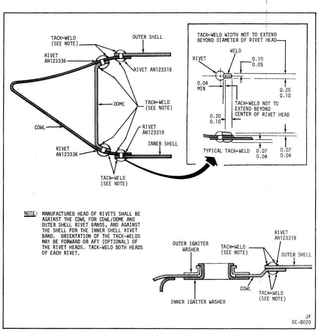
Tack-Welding Combustion Liner Rivet Heads Figure 204
