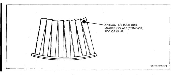
Marking of Stage 6 and 7 Stator Sectors (Typical) Figure 203
