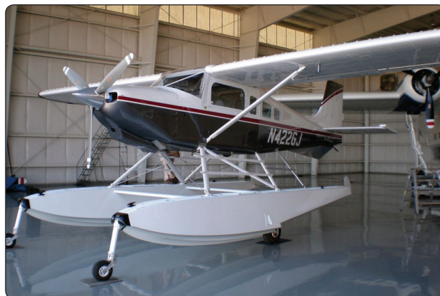
Figure 1-85. Retractable wheels make this aircraft amphibious.
