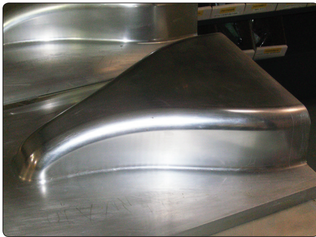
Figure 7-34. A mold of an inlet duct.
