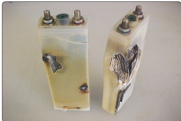
Figure 9-35. Thermal runaway damage.
