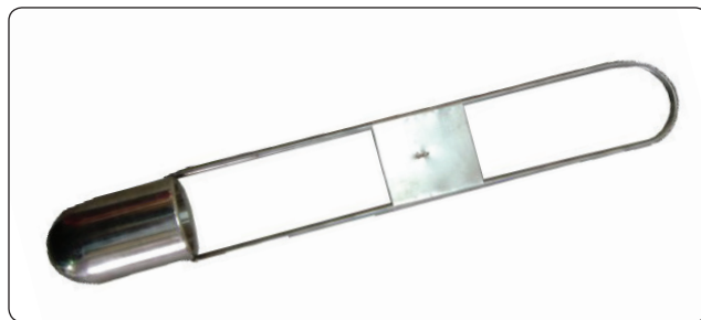
Figure 8-10. A Zahn cup viscosity measuring cup.
