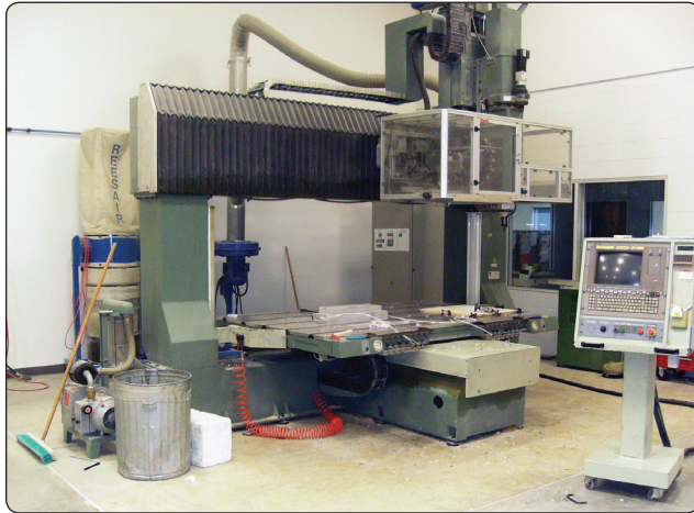
Figure 7-33. Five-axis CNC equipment for tool and mold making.
