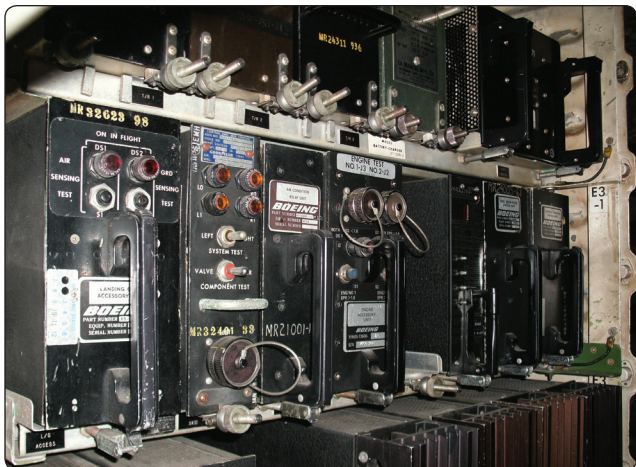
Figure 9-81. Line replaceable units in an equipment rack.
