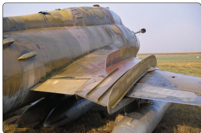
Figure 2-20. Aircraft stall fence.
