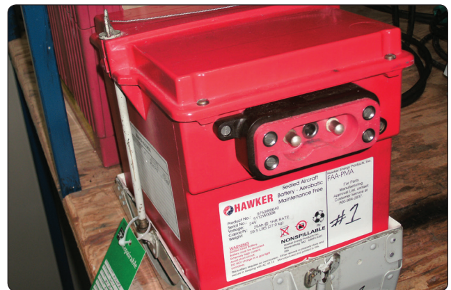
Figure 9-33. Valve-regulated lead-acid battery (sealed battery).
