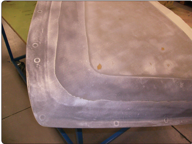
Figure 7-9. Aluminum mesh lightning protection material.
