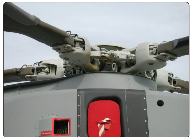
Figure 1-99. Five-blade articulated main rotor with elastomeric bearings.
