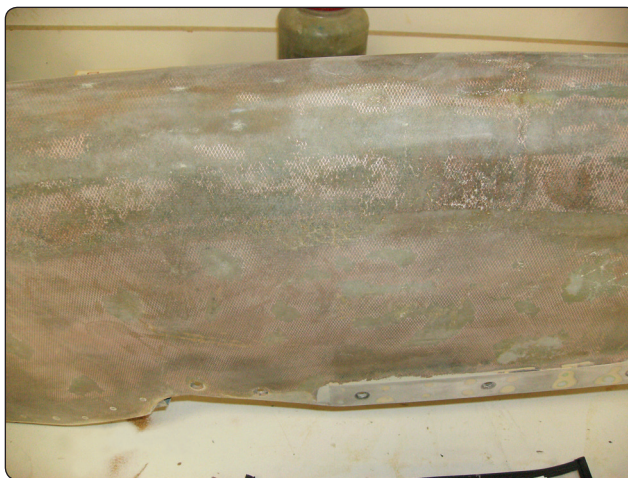
Figure 7-8. Copper mesh lightning protection material.
