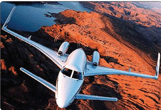
Figure 2-19. The Beechcraft 2000 Starship has canard wings.
