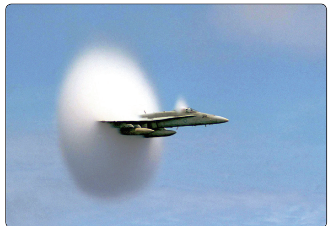
Figure 2-21. Breaking the sound barrier.
