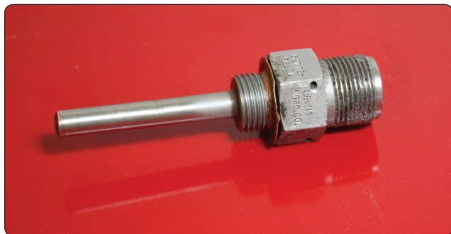
Figure 10-68. An electric resistance thermometer sensing bulb.
