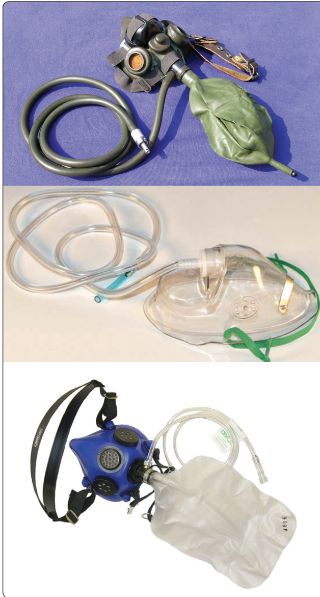
Figure 16-17. Examples of different continuous-flow oxygen masks.
