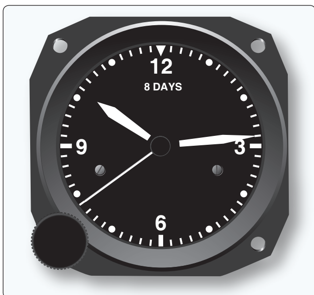
Figure 10-131. A typical mechanical 8-day aircraft clock.
