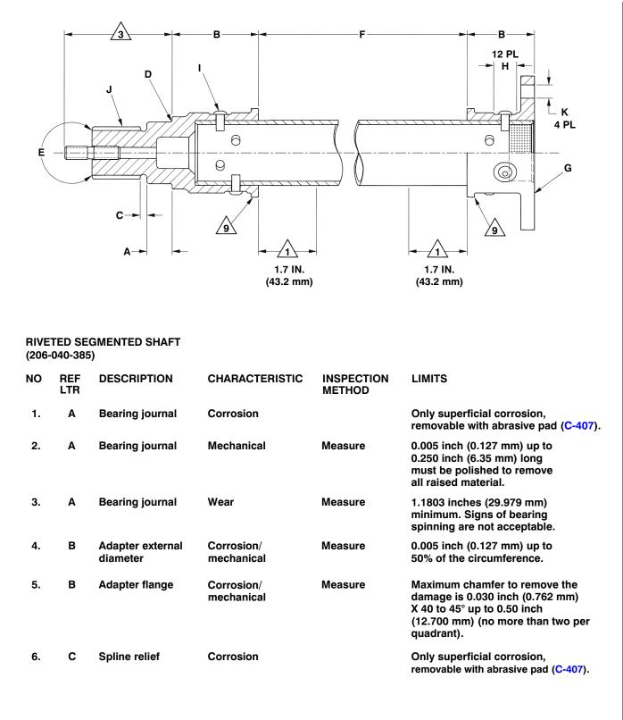
206AB\_MM\_65\_0018a Figure 65-13C. Segmented Tail Rotor Driveshaft (Riveted) — Wear and Damage Limits (Sheet 1 of 3)
