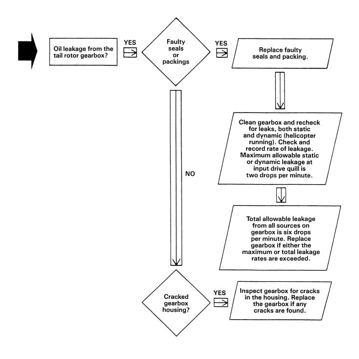
Figure 65-2. Tail rotor gearbox troubleshooting (Sheet 2)
