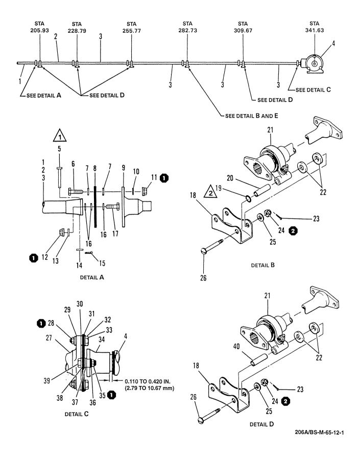
Figure 65-12. Segmented tail rotor driveshafts (Sheet 1 of 2)
