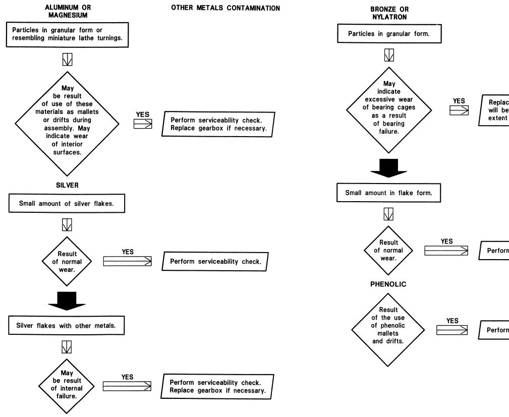
Figure 65-4. Corrective action for contamination found in tail rotor gearbox (Sheet 2)
