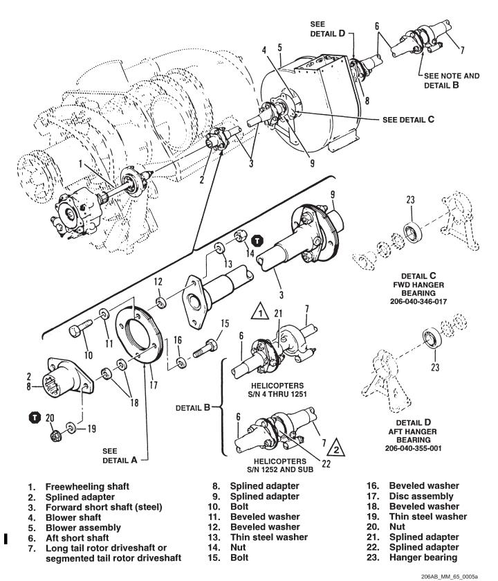
Figure 65-6. Forward and Aft Short Tail Rotor Driveshafts (Sheet 1 of 2)
