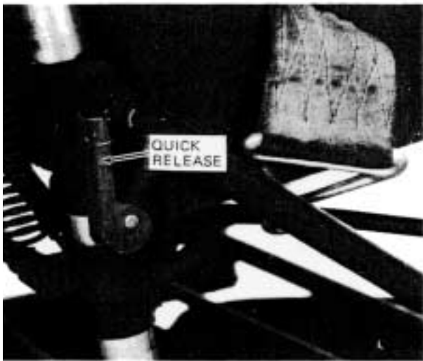
Figure 2-48. Crew armored seat reclining quick release
