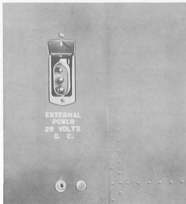
Figure 7-5. External Power Receptacle
