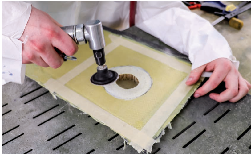
Figure 9-2-9. Mechanical sanding with a right angle sander gives more control. Sanding with too much pressure, or too coarse of grit sandpaper are common problems. It can be difficult to see where one layer stops and the next starts, resulting in damage to the core.
