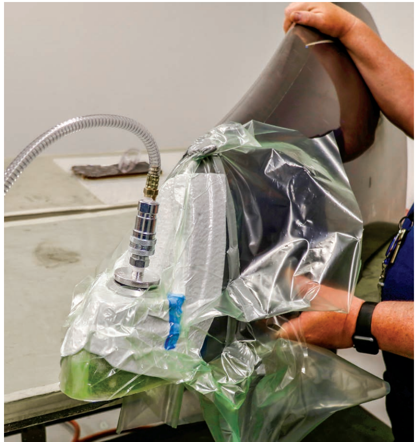
Figure 10-3-2. Vacuum hose used for vacuuming in an area where the temperature does not go above room temperature, the internal wires to prevent collapsing can be seen in the clear tubing. The vacuum valve is a quick connect style.
