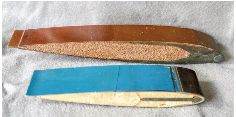
Figure 4-3-4. Polyurethane foam cores used with fiberglass skins shown in a cross section of Bell 49 helicopter blades.
