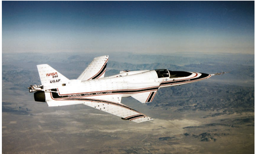
Figure 2-7-5. The X-29 was constructed with composite materials in the wings. Courtesy of NASA
