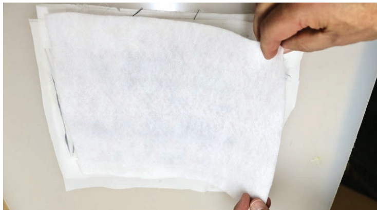
Figure 7-2-4. The bleeder/breather material is placed over the peel ply to absorb extra resin and allow air to flow throughout the repair.
