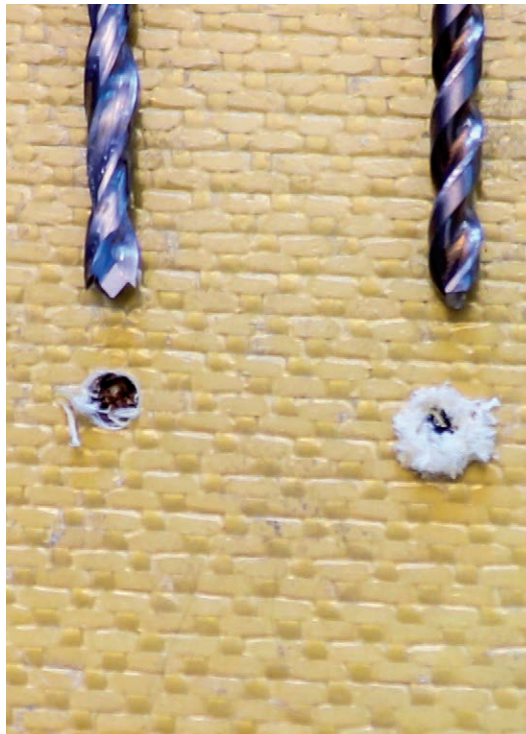
Figure 9-2-4. Special brad point drills are made for drilling aramid composites. The hole on the left is cut with a brad point bit, as compared to the hole on the right, cut with a standard sheet metal bit.
