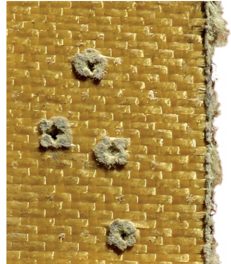
Figure 2-2-2. Cutting or drilling aramid can leave a fuzzy edge, which can lead to problems.
