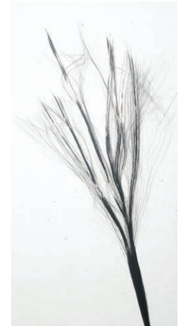
Figure 2-8-1. A bundle of carbon fiber filaments make a tow.
