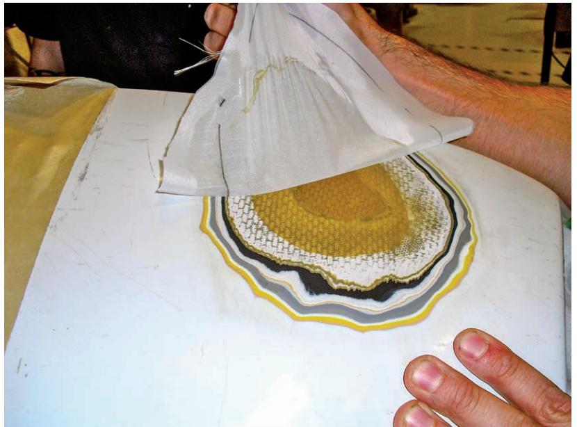
Figure 12-7-13. After removing the vacuum bagging materials and the splash mold, the peel ply is removed, and the repair is finished, except for painting.
