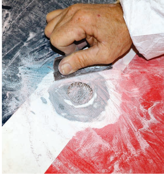
Figure 9-2-8. Composite layers are very thin, and hand sanding the paint away from the repair prevents going through the structural composite layers.
