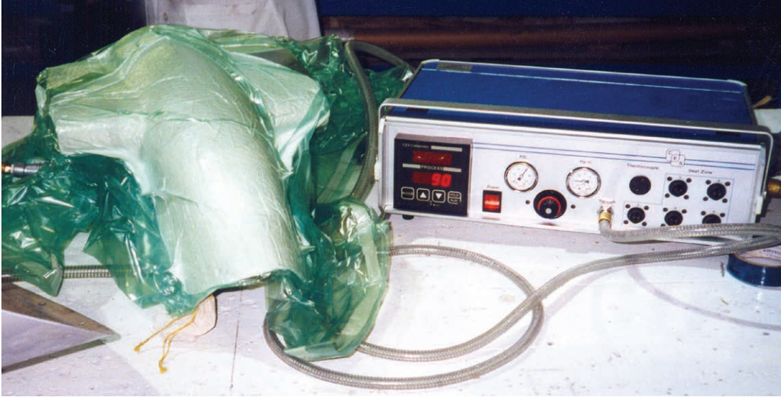
Figure 7-5-1. To prevent the part from collapsing in any area, the entire part is put into a self-enclosing bag. The bag must be made about three times larger than the part to allow extra bagging film to contour around the part on the inside and outside, giving the proper amount of pressure on both sides of the part.
