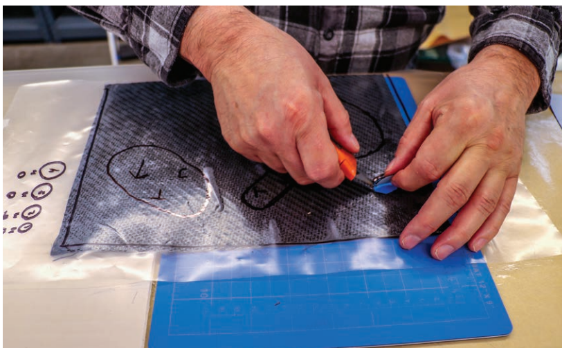
Figure 11-5-28. The clear plastic that was used to outline the size and orientation of the patches is placed over the pre-preg material, and cut out with a razor knife or scissors.
