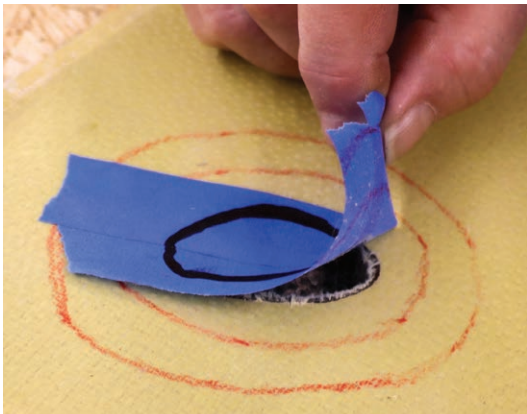
Figure 11-5-15. Mark the routed out area on the tape to get the size needed to replace the core.
