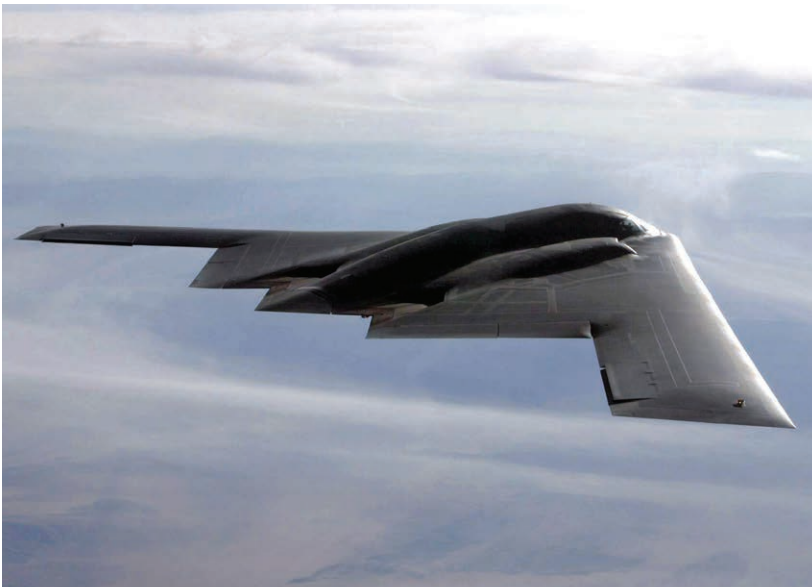
Figure 1-2-7. The B-2 incorporates the flying wing construction to help in its stealth capabilities.
