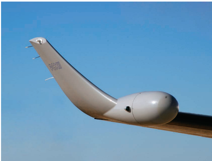
Figure 3-1-4. Radomes house radar equipment and are made of polybutadiene resin composites.
