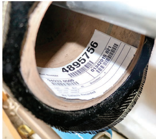
Figure 10-4-1. A sticker might be on the inside of the roll that corresponds to paperwork that is sent with the fabric.
