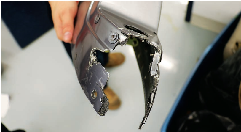
Figure 11-5-5. Repairs are not always circular. The half inch per ply around the edges is still required. This part was repaired using a splash mold.
