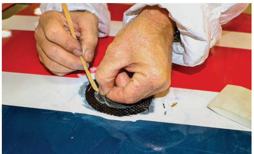
Figure 11-5-27. Once the patch is in place, carefully remove the plastic on the top of each patch. Use a tool such as a mixing stick to hold the patch in place while removing the plastic.
