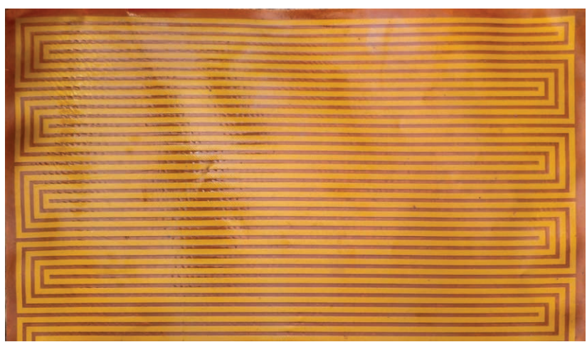
Figure 8-3-4. Fine wires are imbedded in the heat blanket and are controlled by a hot bond unit.
