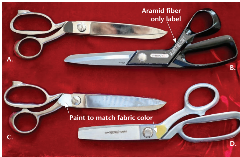
Figure 9-1-1. The scissors on the left (A and C) are standard fabric scissors marked with black and white paint. They also work well on any of the vacuum bagging materials. The scissors on the right (B and D) are for aramid only and are solid ceramic blades that are serrated. The black handled ones have "Aramid fiber only" engraved on them. The blunt tip scissors (D) are also serrated and marked with yellow paint.
