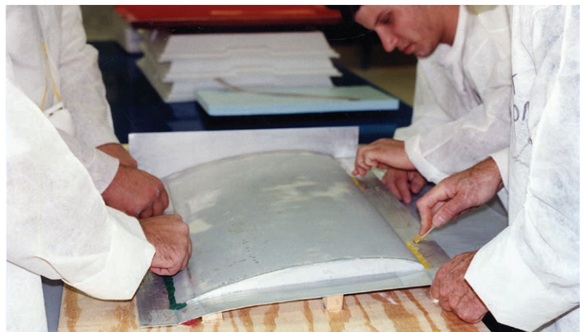
Figure 5-3-4. Building the parting board around the plug. The mold is made in two parts on the top side and the bottom side of the plug.
