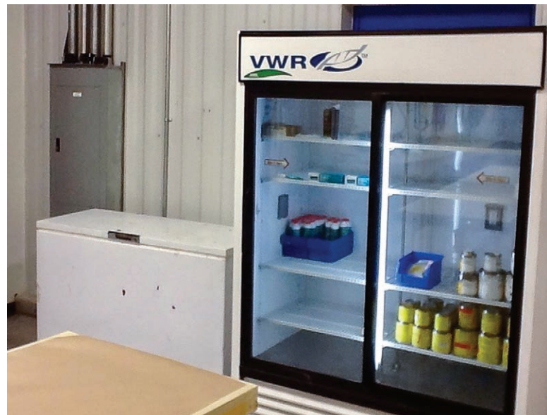
Figure 10-1-2. A chest freezer, on the left, is used for storing pre-preg materials, and a refrigerator for storing some adhesives and chemicals is on the right.
