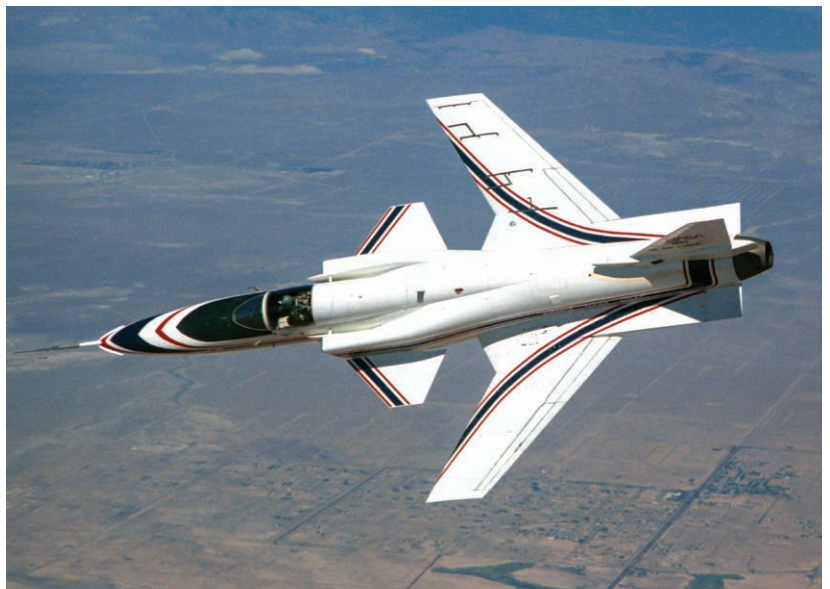
Figure 1-2-5. The composites used in the forward-swept wing design of the X-29 withstand extraordinary stresses. Courtesy of NASA
