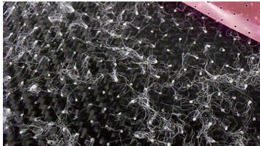
Figure 7-2-2. The fuzz of the bleeder stuck to the final part. This needs to be sanded out.
