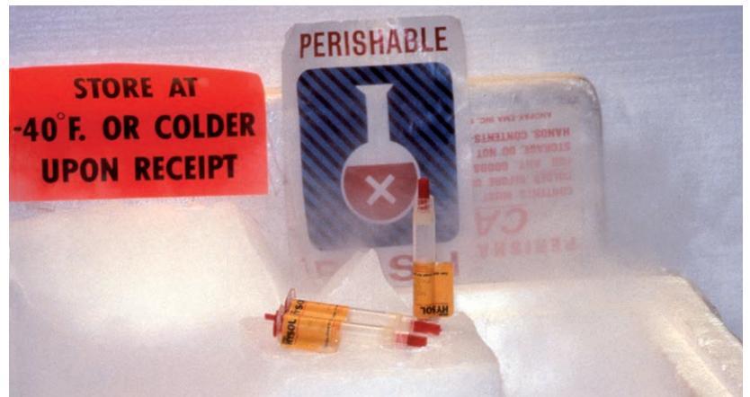
Figure 6-4-2. Some materials require specific storage temperatures. Note that the packaging statement, "Store at -40°F. or colder upon receipt," actually means below 40° and not 40 below 0°.
