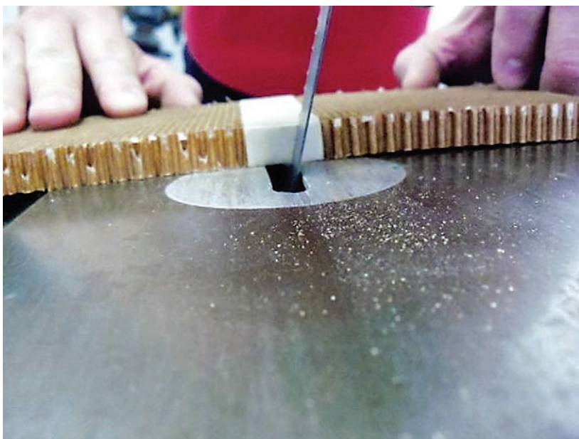
Figure 9-2-15. Special bandsaw blades are available for cutting carbon/graphite material. Some fuzzing is produced when cutting aramid, but it can be cleaned up by hand.
