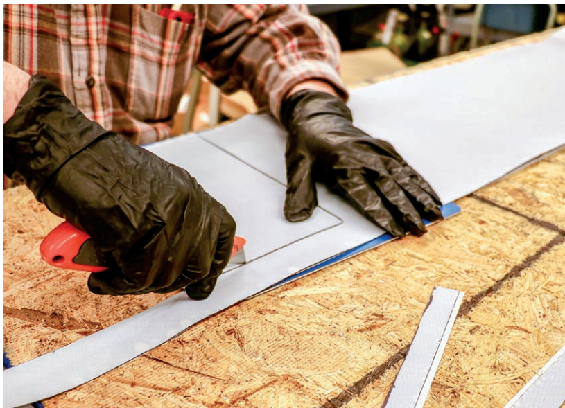
Figure 9-1-2. Cutting pre-preg composites with a razor knife.
