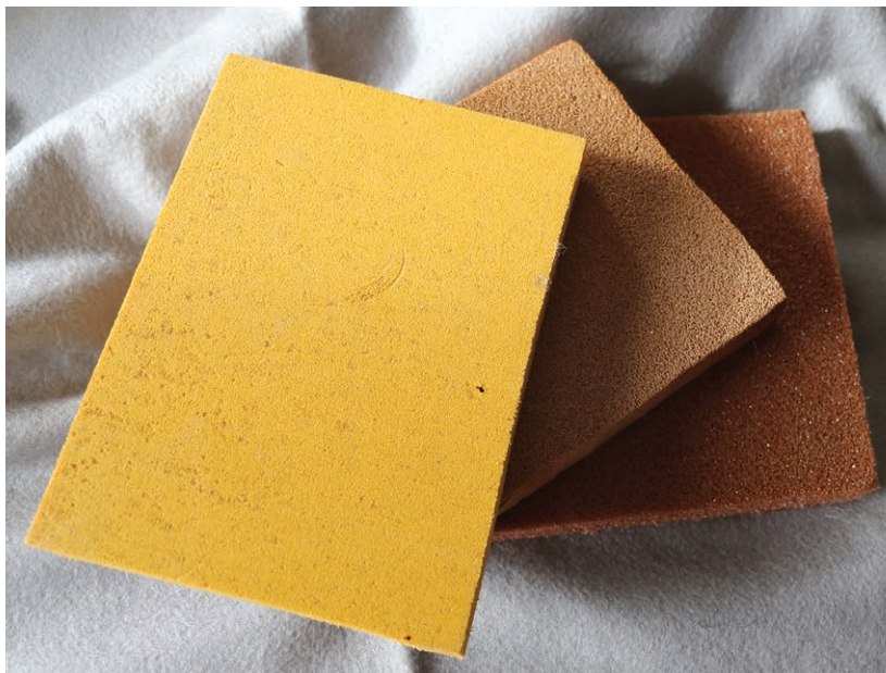
Figure 4-3-1. Foam cores for sandwich construction can be Styrofoam, urethane, polyvinyl chloride, or Strux (cellulose acetate).
