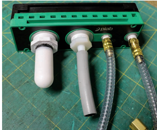
Figure 10-3-1. Vacuum is created by using compressed air through a series of venturi tubes.
