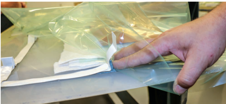
Figure 7-3-6. The vacuum bag film goes up one side of the pleat and down the other.
