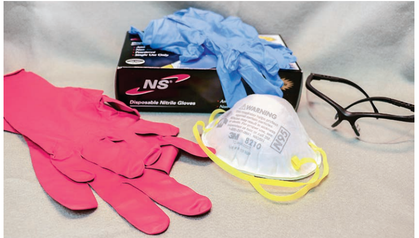
Figure 6-2-1. Safety gloves, goggles, respirator, and dust masks are required when working with composites.
