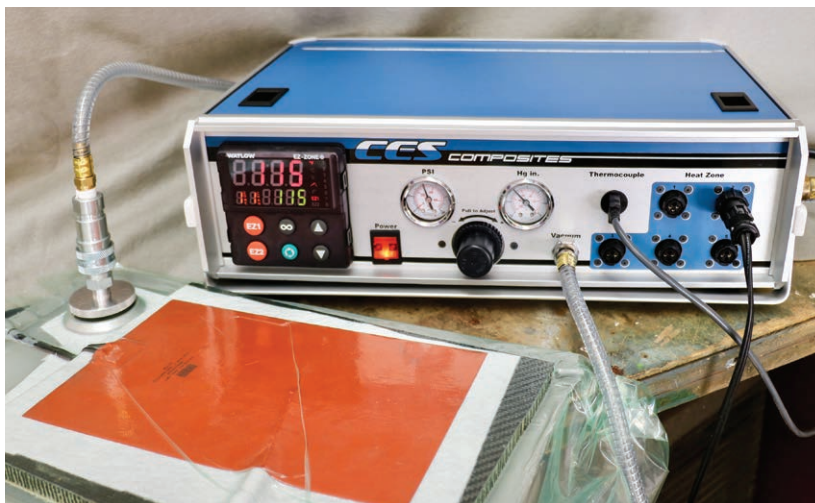
Figure 8-3-1. Hot patch bonding is done with a heat blanket and is normally used with a vacuum bag. Controller devices are used, and the temperatures and times should be recorded.
