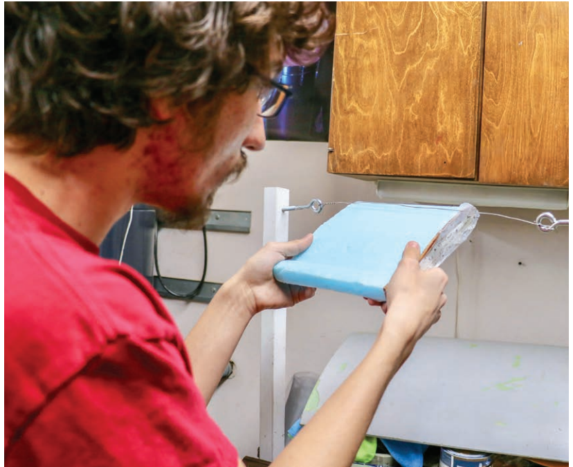
Figure 4-3-3. Using a hot wire cutter around a template to shape Styrofoam.
