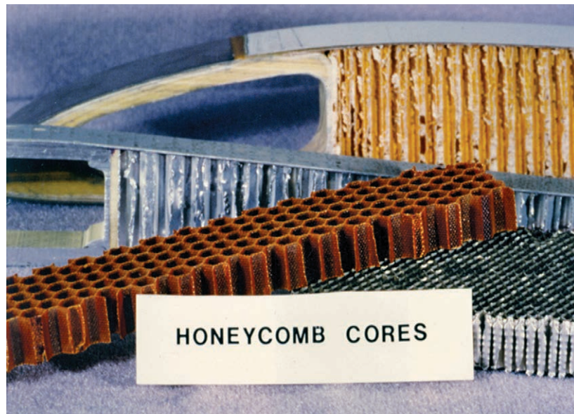
Figure 4-2-1. Typically, honeycomb cores used in aircraft construction are made of aluminum or Nomex.
