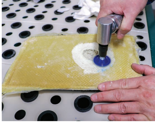
Figure 11-5-7. Sanding is the method that is usually used to remove the plies with the most control.
