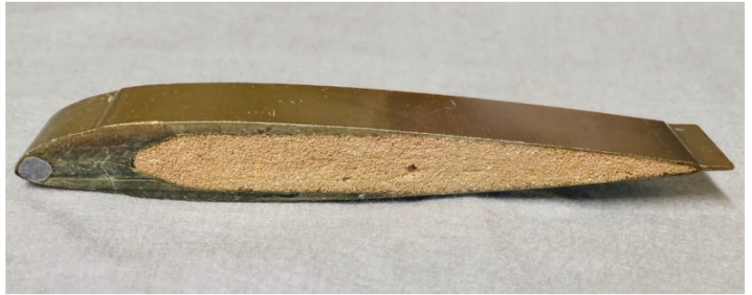
Figure 3-1-2. This cutaway of a rotor blade uses fiberglass with epoxy resin skins, bonded to a urethane core with metal bonded into the leading edge.
