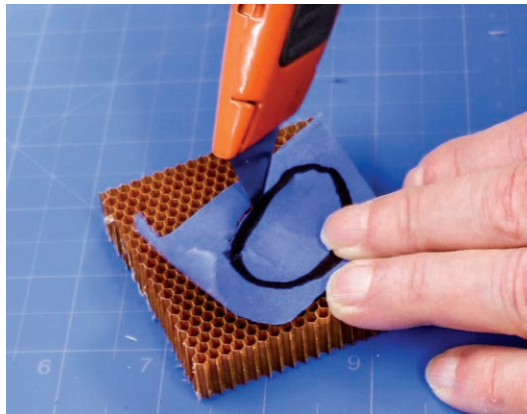
Figure 11-5-17. Cutting out the new honeycomb plug.
