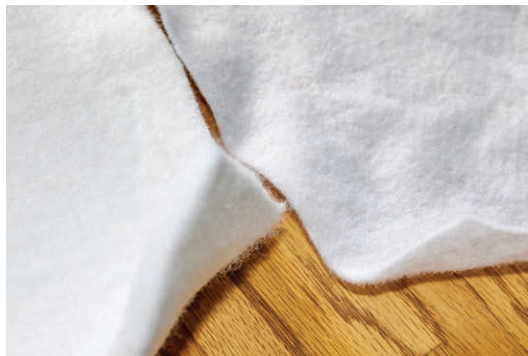
Figure 7-2-3. The 10-oz. bleeder (left) is very thick (1/4-in. thick) and will pull more resin out than the 4-oz. (right), which is thinner (1/8-in. thick).
