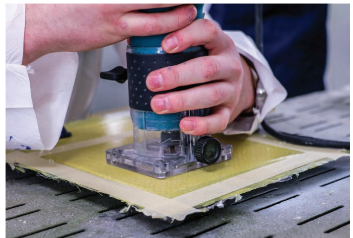
Figure 11-5-6. A right-angle grinder (left) fitted with a router bit can be used to clean out the damaged honeycomb core. A trim router (right) is used to remove the core with a flush bit. A diamond cut bit is used to prevent damage to the honeycomb while routing.
