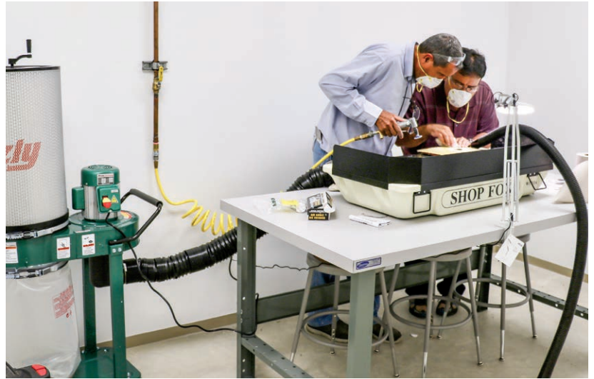
Figure 10-1-6. Downdraft tables are used to pull the fine dust from the air.
