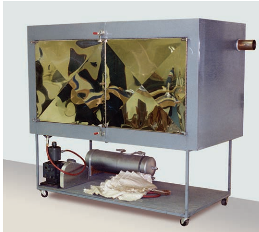
Figure 8-3-9. Oven curing is often used in the manufacturing process to cure many parts at the same time.
