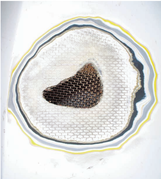
Figure 12-7-9. The damaged honeycomb has been removed, and the fiber layers have been sanded down.
