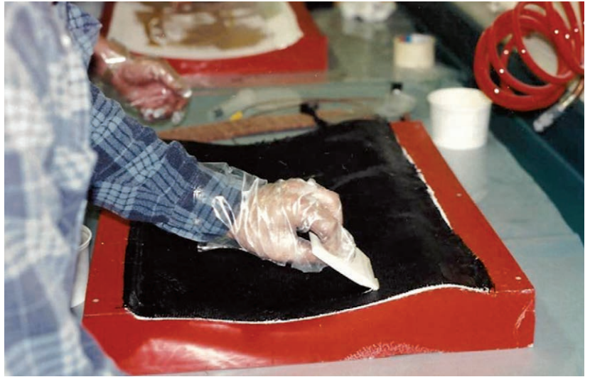
Figure 5-3-6. Laying fabric into the mold.
