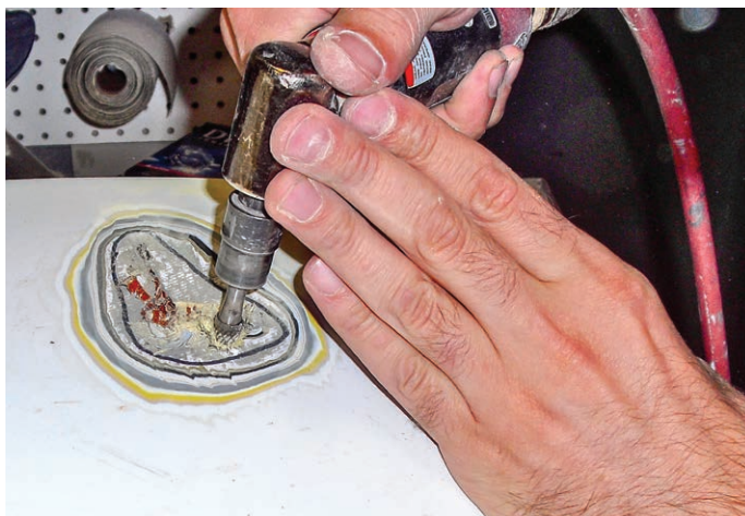
Figure 11-5-6. A right-angle grinder (left) fitted with a router bit can be used to clean out the damaged honeycomb core. A trim router (right) is used to remove the core with a flush bit. A diamond cut bit is used to prevent damage to the honeycomb while routing.
