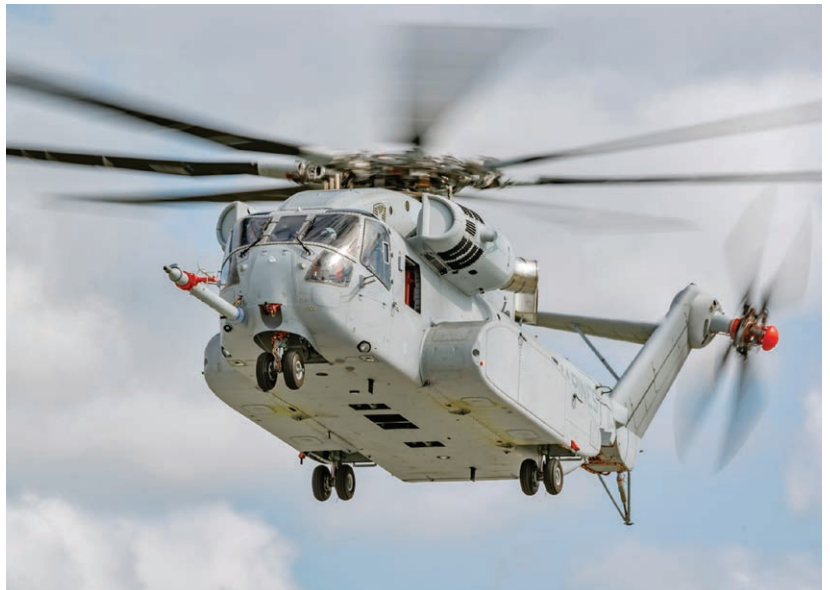
Figure 1-2-4. The Sikorsky CH53K has a 70 percent composite airframe.
