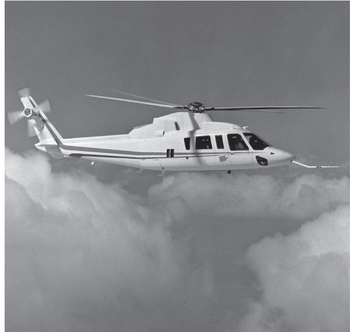
Figure 1-2-2. The S-76 horizontal stabilizer is made of Kevlar and Nomex honeycomb.
