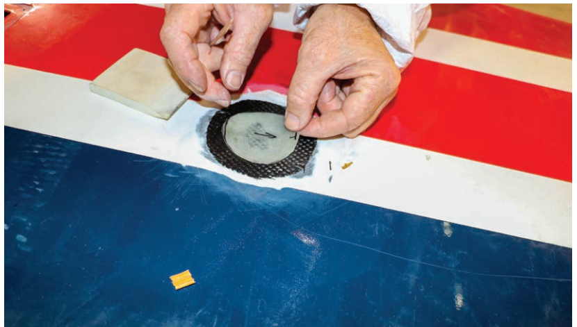
Figure 11-5-26. Remove the back plastic and match the orientation of the fiber patch with the orientation designated in the SRM for each patch.
