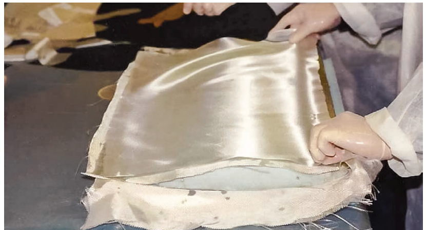
Figure 5-3-3. Two layers of fiberglass are placed on the foam to make a plug.
