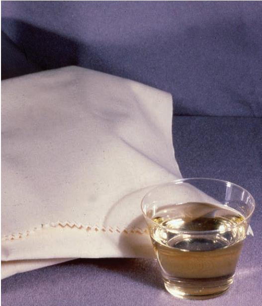
Figure 1-1-2. Dope and fabric is a type of composite material that is still in use today.
