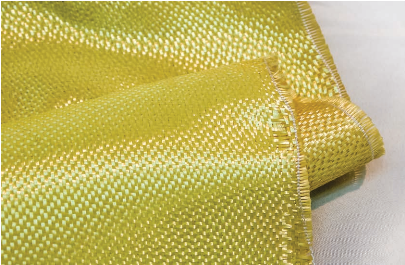
Figure 2-2-1. Aramid fibers can be woven by different weavers, but DuPont's Kevlar is probably the most well known because DuPont was the first to manufacture it. It has a tensile strength roughly four times that of aluminum alloy.
