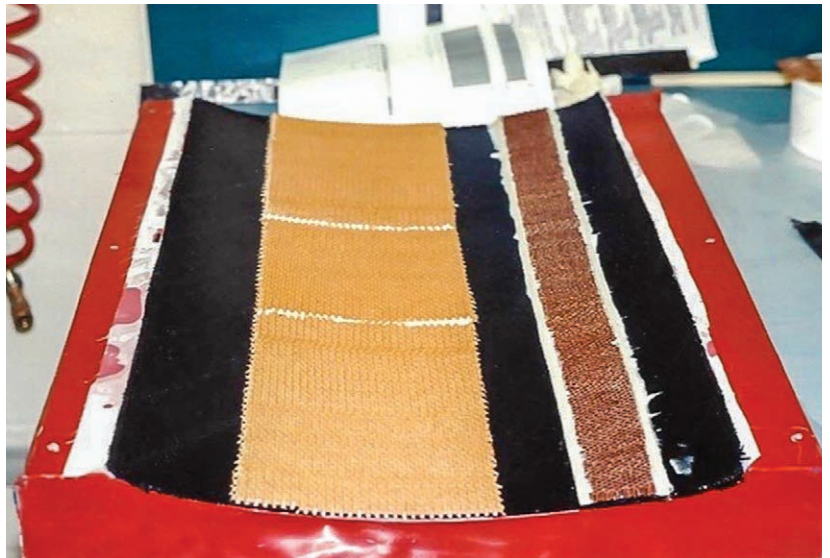
Figure 5-3-7. Any honeycomb is added, then another final piece of the fabric is added over the honeycomb.
