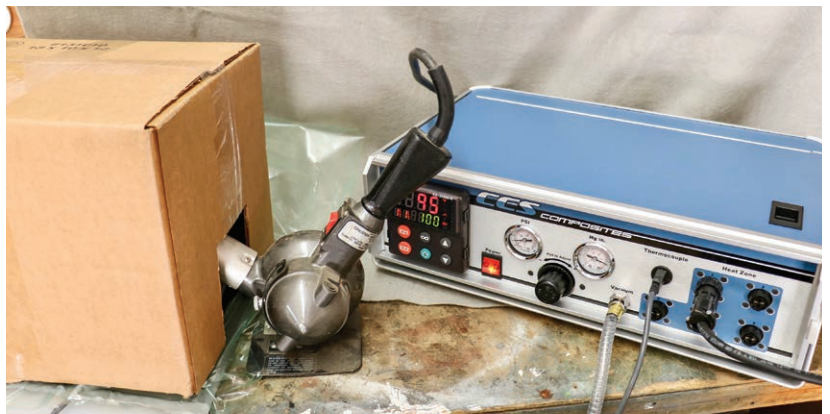
Figure 8-3-7. A heat gun is used with a controller to cure a curved part to which a heat blanket cannot conform to the shape. Here, a box is used to keep the heat in (150°F max for cardboard).
