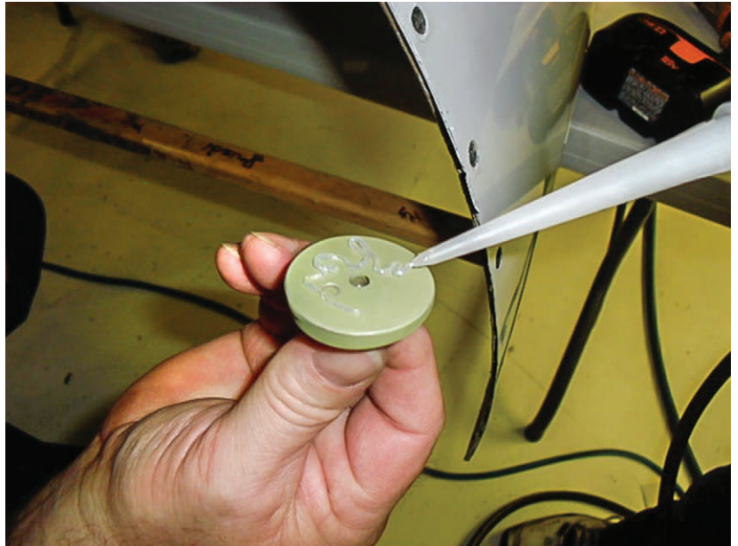
Figure 3-2-3. Dispensing the mixed resin through a syringe.
