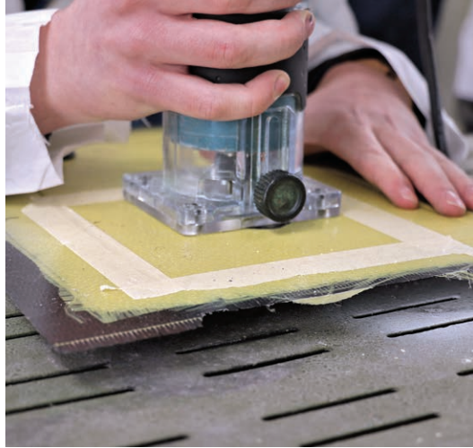
Figure 9-2-11. Standard routers, or trim routers with speeds of 25,000 to 30,000 r.p.m., work well for cutting composites. Using special bits designed for specific materials normally produces good results to remove honeycomb cores.
