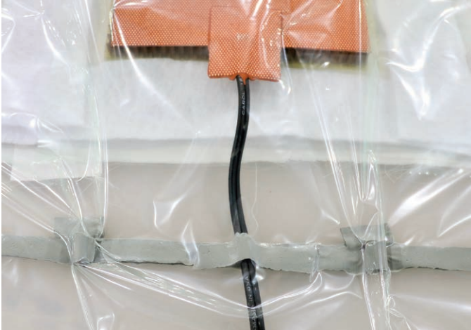
Figure 7-3-3. Place the heat blanket wire over the sealant tape, and then place another small piece of sealant tape over the wire to prevent air from leaking around it.
