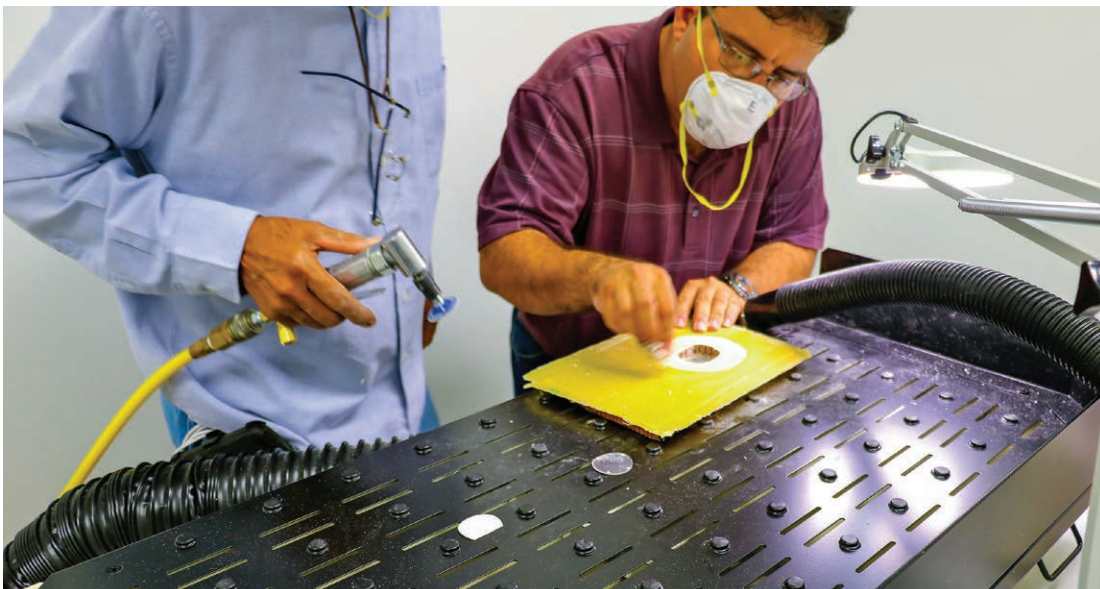
Figure 6-5-1. Machining or sanding composite structures on a downdraft table reduces airborne particles.
