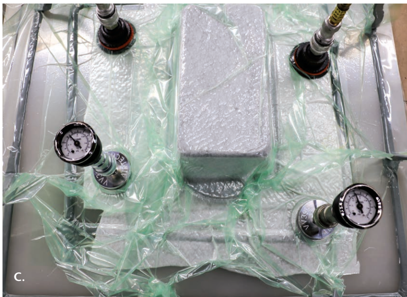
Figure 7-5-4. (A) The part is vacuum bagged, and a metal cage is placed over the part. (B) Breather material and a second vacuum bag are added. (C) Vacuum is pulled on the inside vacuum bag and the outside vacuum bag. No additional vacuum is gained.
