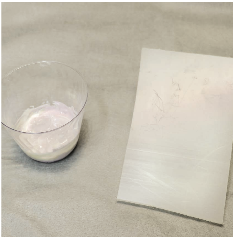
Figure 3-1-1. When the resin is mixed with a catalyst or hardener, it is in a liquid form. After curing, it is a solid plastic. In composite use, the mixed resin is combined with a fiber reinforcement to form a fiber-reinforced plastic.
