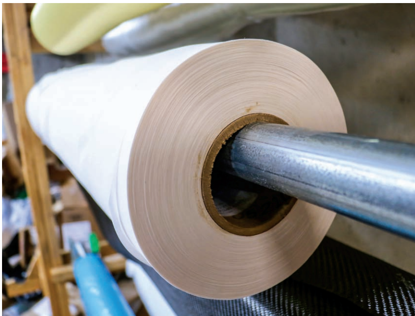
Figure 10-0-1. Most materials come from a supplier or weaver in very large quantities. This roll of peel ply has more than 700 yards on it.
