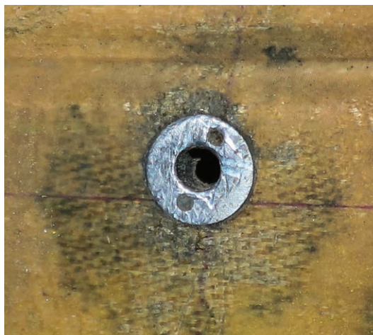
Figure 9-3-4. Inserting a fastener into a sleeve like this reduces damage to the laminate.
