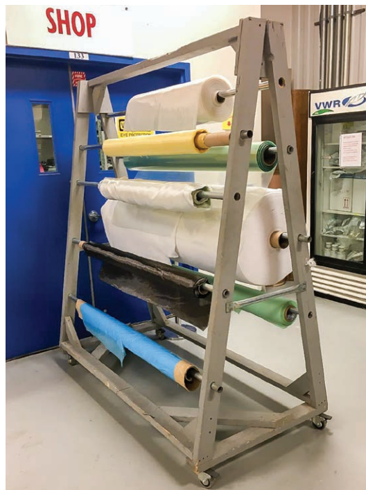
Figure 10-1-3. Composite fabrics and vacuum bagging materials stored on a rack help maintain cleanliness and safety.
