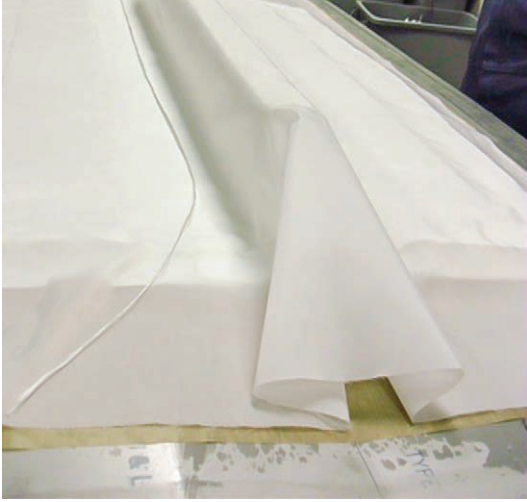
Figure 5-2-6. Fabric is laid into the mold, a 6-in. spar is placed at a 90° angle, followed by the final layers of fabric over the entire structure. Peel ply is draped over the entire structure. This part will be vacuum bagged.
