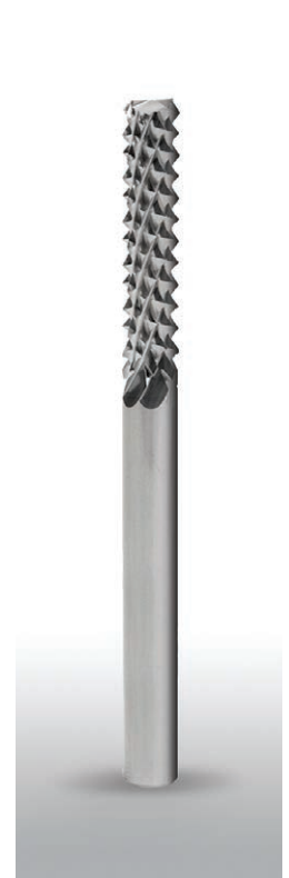
Figure 9-2-12. A diamond-cut router bit is used to clean out the honeycomb core without tearing the edges of the honeycomb.
