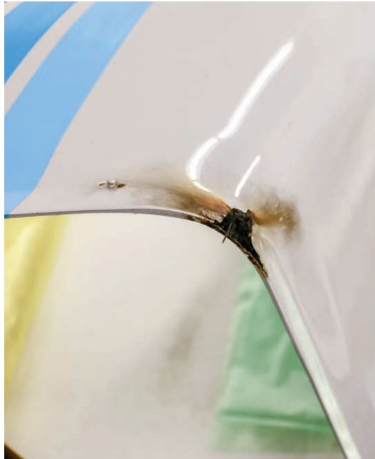
Figure 11-6-1. Lightning strike damage.
