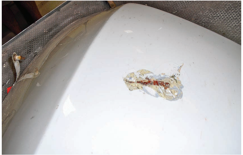
Figure 12-7-5. Damage to the part goes through the top two layers of Kevlar, into the core, and one layer below the core.
