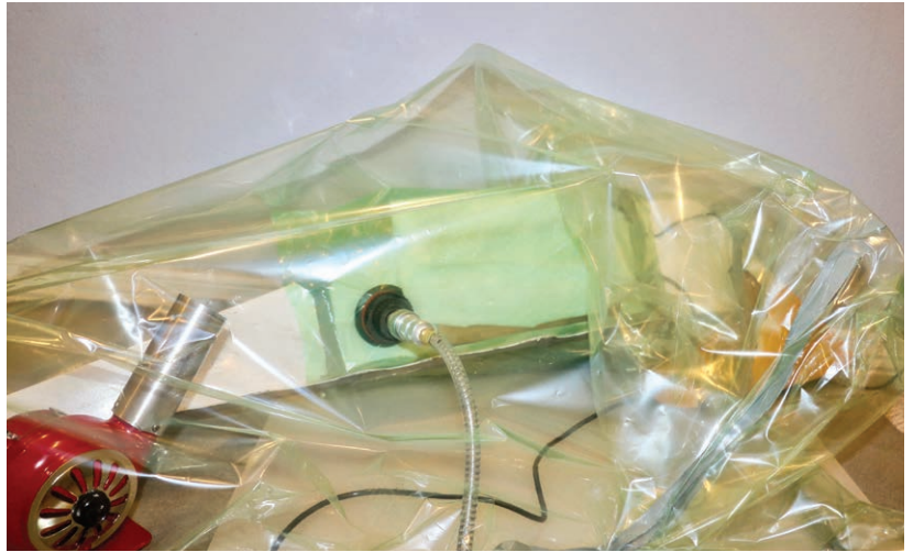
Figure 8-3-6. The repair is vacuum bagged, then an outer bag is placed around the repair area. This forms the tent to hold in the hot air. The heat gun blows air up toward the top of the bag. There is a thermocouple at the repair site, and the heat gun is plugged into the controller. With the ramp and soak feature, the heat gun follows the program.
