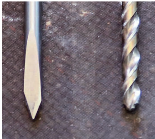
Figure 9-2-6. A spade bit cuts more with its outer edge; the inner portion mostly removes waste material. Traditional spade or dagger bits with an included angle of 118^\circ are used in PLEXIGLAS ® windshields. For composite work, the more pointed bit with an included angle of 60^\circ is used.
