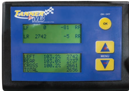
Figure 7-1-4. The scale shows a weight of 2,742 lbs. This is the weight on the part. Vacuum bagging gives a great amount of pressure.
