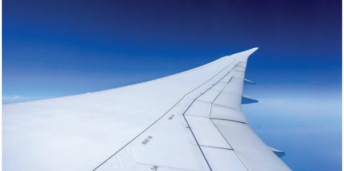
Figure 3-1-3. The wing on a Boeing 787 uses a flexible type of epoxy resin reinforced with carbon fiber to be flexible in flight.
