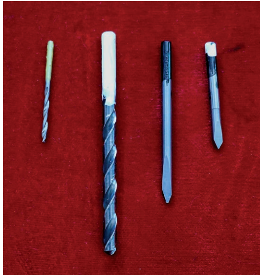
Figure 9-2-1. Bits are painted for the type of fabric they are used on. The yellow paint on the left bit is for aramid, the white, fiberglass, and the black for carbon. The bit on the right was originally used for carbon, but as it dulled, white paint was added to show it would be a good bit for hybrid carbon/fiberglass components.
