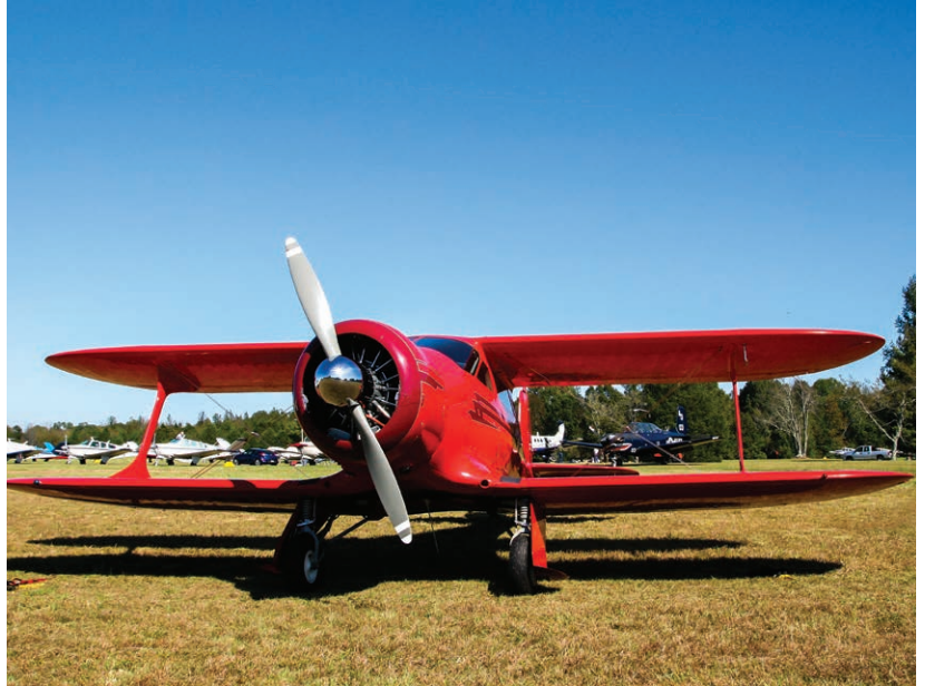
Figure 1-1-3. Dope and fabric cover the Beech Staggerwing fuselage and wings.
