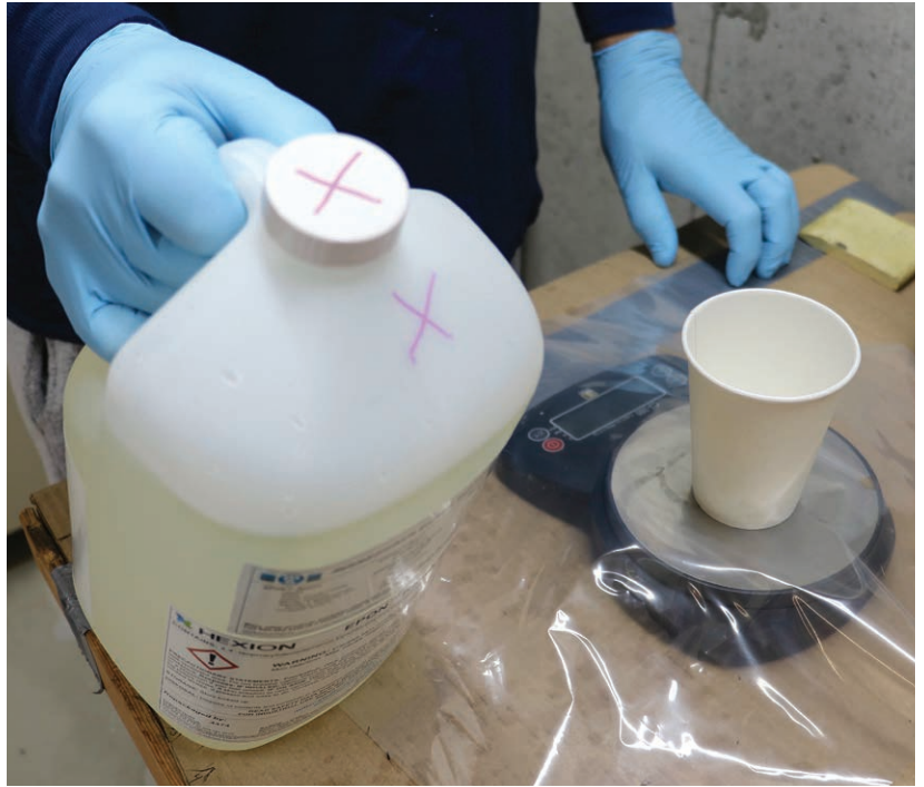
Figure 3-2-1. Scales are used to accurately measure the mix ratio for a resin system.
