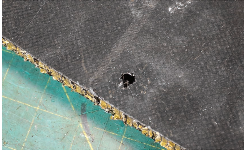
Figure 9-2-5. Carbon can break during drilling, causing the hole to be larger than that of the drill bit.
