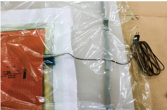
Figure 7-3-4. Place the thermocouple under the heat blanket, place the wire over the sealant tape, and affix a second piece of sealant tape over the wire to prevent air from leaking around it.
