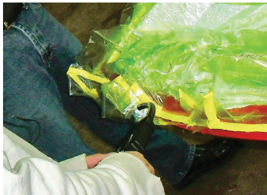
Figure 7-3-7. Here, an ultrasonic leak detector is used to find a leak in the vacuum bag. It amplifies the hissing sound in areas where loud noises are a problem.
