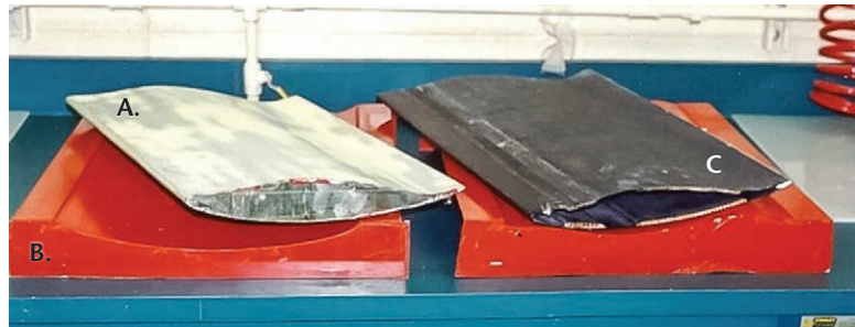
Figure 5-3-1. This photo shows a sample plug (white), mold (red), and a finished component (black).
