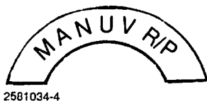
Located at Upper RH Switch Control Wheel Pilot and Copilot Aircraft 35-002 thru 35-172, 36-002 thru 36-041 Incorporating AAK 70-3 Control Wheel Kit, Pilot and Copilot and Modified by AMK 80-13 Control Wheel Switch Identification Collars and Placards
