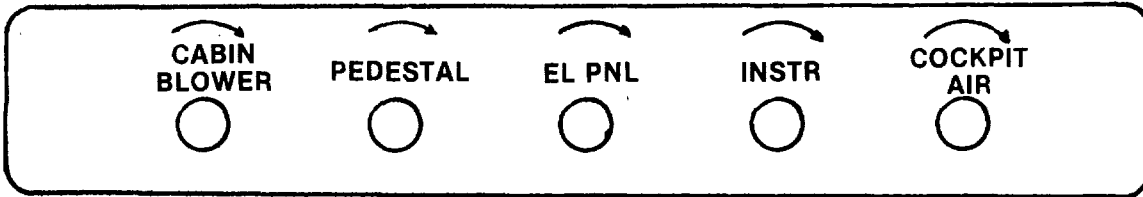
Located on Pilot's Dimmer Control Panel (Grey) Panel Includes CABIN BLOWER and COCKPIT AIR Provisions
