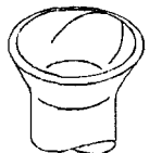
SCRATCHES/GROOVES- INTERNAL LONGITUDINAL OR SPIRAL
