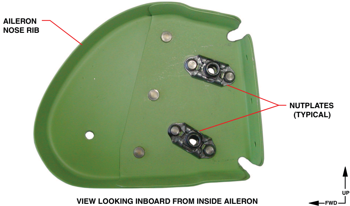
Aileron Hinge Nose Rib Nutplates Figure 6
