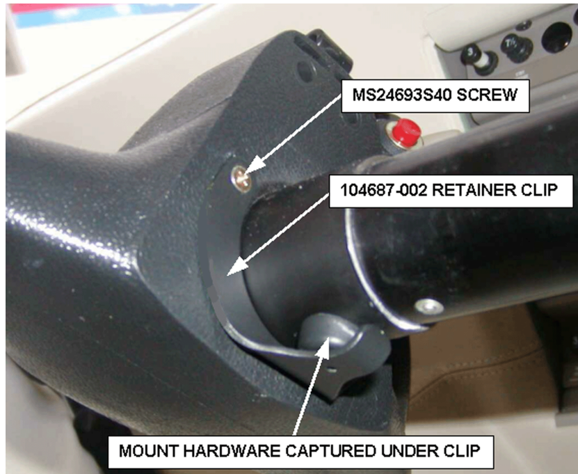
Control Wheel Installation Figure 1
