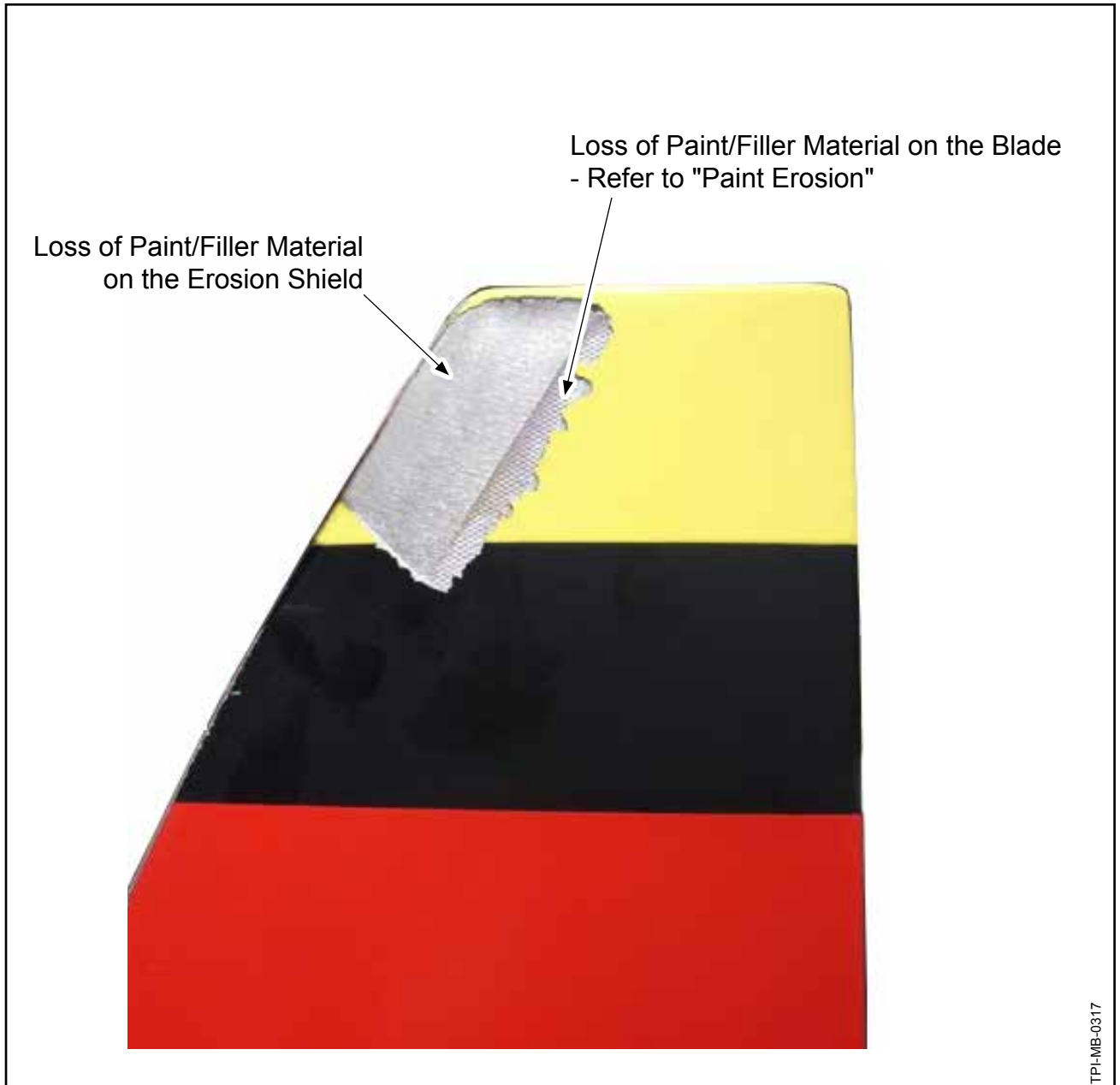
Erosion Shield: Loss of Paint/Filler Material Figure 2-5
